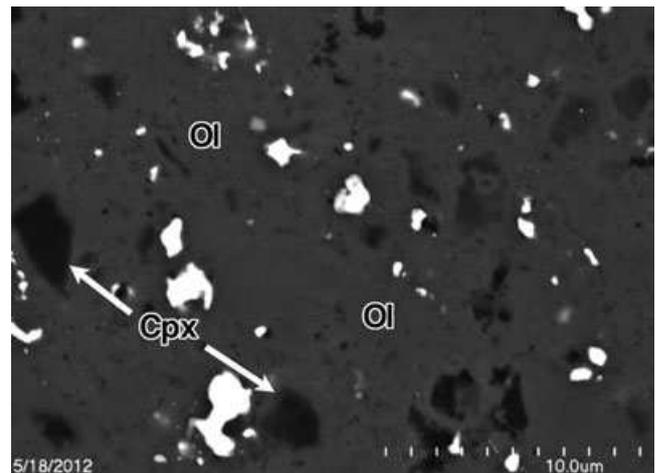
Fig. 8. Backscattered electron image of a matrix area in Y-82094 (111-1). The dominant phase is olivine, showing a sintered texture, with minor Ca-rich pyroxene (Cpx). Bright grains are mostly Fe-Ni metal.
