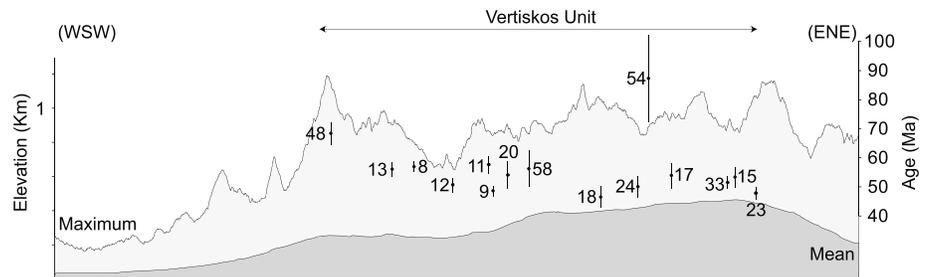
**Figure 5.** WSW-ENE trending swath elevation profile of the Chalkidiki Peninsula extracted from the ASTER Global DEM v2. The profile stretches from the Vardar-Axios basin to the Strymon basin (see Figure 1). The AFT ages for the samples used for the joint profile modeling approach are plotted, and the corresponding calculated apatite FT ages are read on the right vertical axis.
