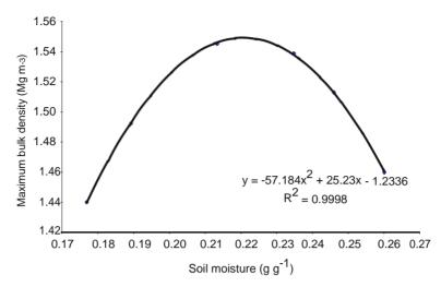
Fig. 9.2 Characteristics of the Proctor compaction curve
