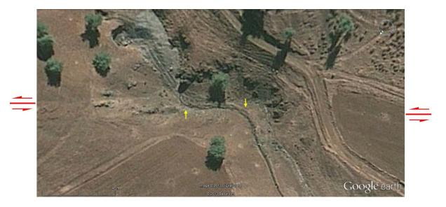
At this site (Fig. 9) a small stream flows down a bluff within the Hatay ophiolite, crossing the fault from the southeast. The stream, incised into a young alluvial fan, is offset leftward (between points CA 03441 94841 and CA 03413 94817) in line with the foot of the bluff, providing evidence (equivalent in character to similar evidence documented at sites along the Amanos Fault by Karabacak et al., 2010) of a component left-lateral slip. The left-lateral offset between these points is
