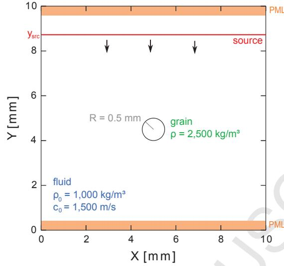
Figure 3: Scheme of the experiment with 1 grain
