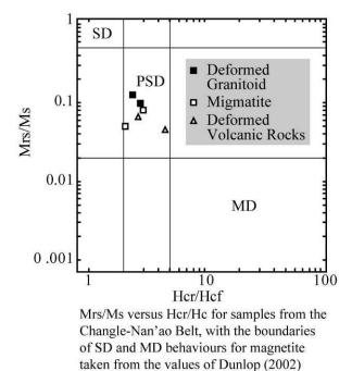
Figure 8. Day-plot diagram of measured samples of the Changle-Nan'ao Belt to define the magnetite size. Mrs: saturation remanence, Ms: saturation magnetization, Hcr: remanent coercive force Hcf: ordinary coercive force, SD: single domain, PSD: pseudo-single domain, MD: multi-domain.
