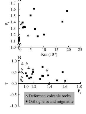
Figure 9. AMS scalar parameters for each site and main lithologies. A:  $P_J$  (corrected anisotropy degree) vs. Km (mean bulk magnetic susceptibility in  $10^{-3}$  SI); B: T (shape parameter) vs.  $P_J$  (corrected anisotropy degree). The calculations of T and  $P_J$  can be found in Jelinek (1981).
