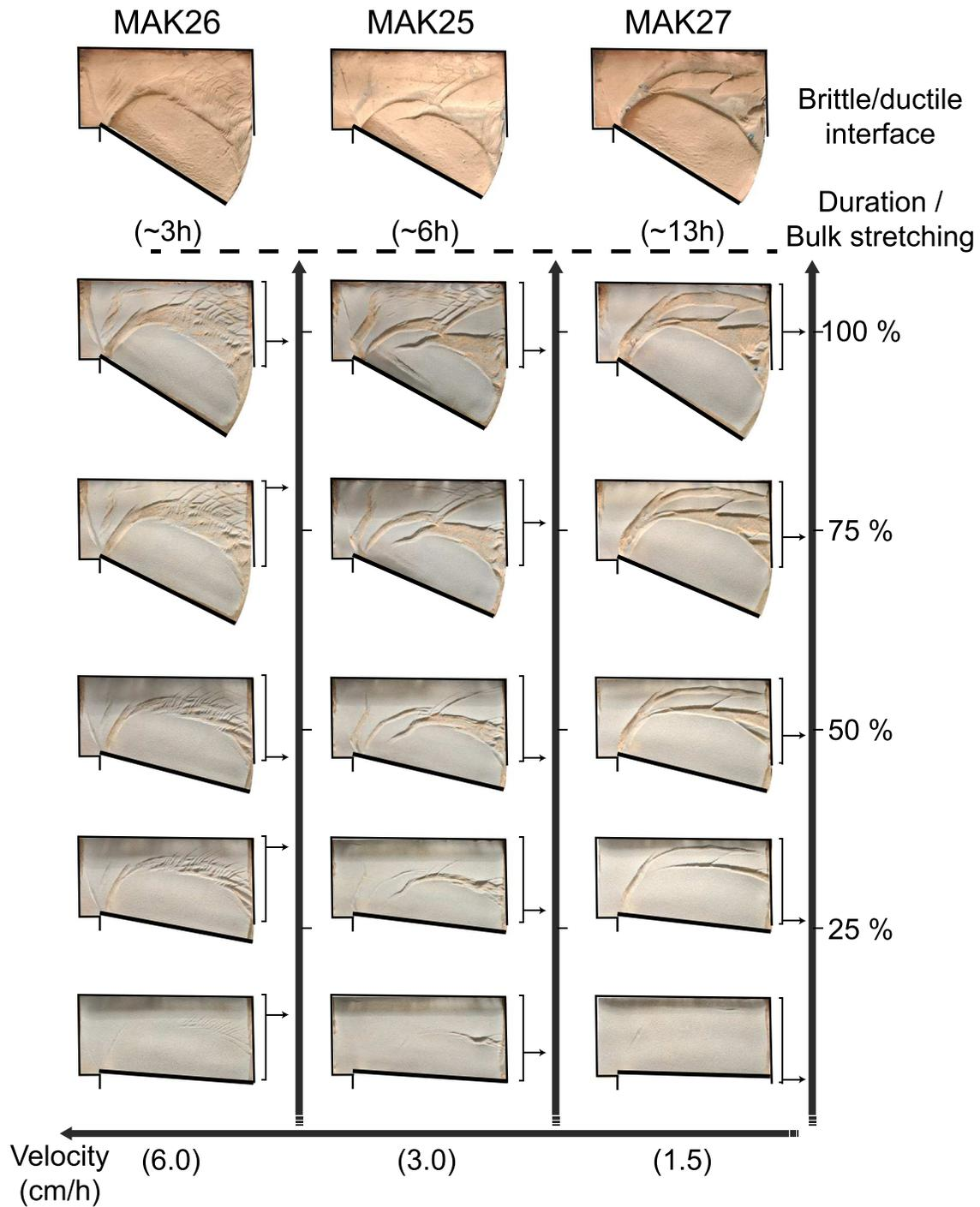
**Figure 8.** Selected top-view snapshots for Setup A experiments (thicker sand layer; see Figure 6) using three tested displacement velocities. The brittle-ductile interface at the end of each experiment is also shown at the top. To facilitate the discussion, a virtual north is taken as facing upward. See text for details.
