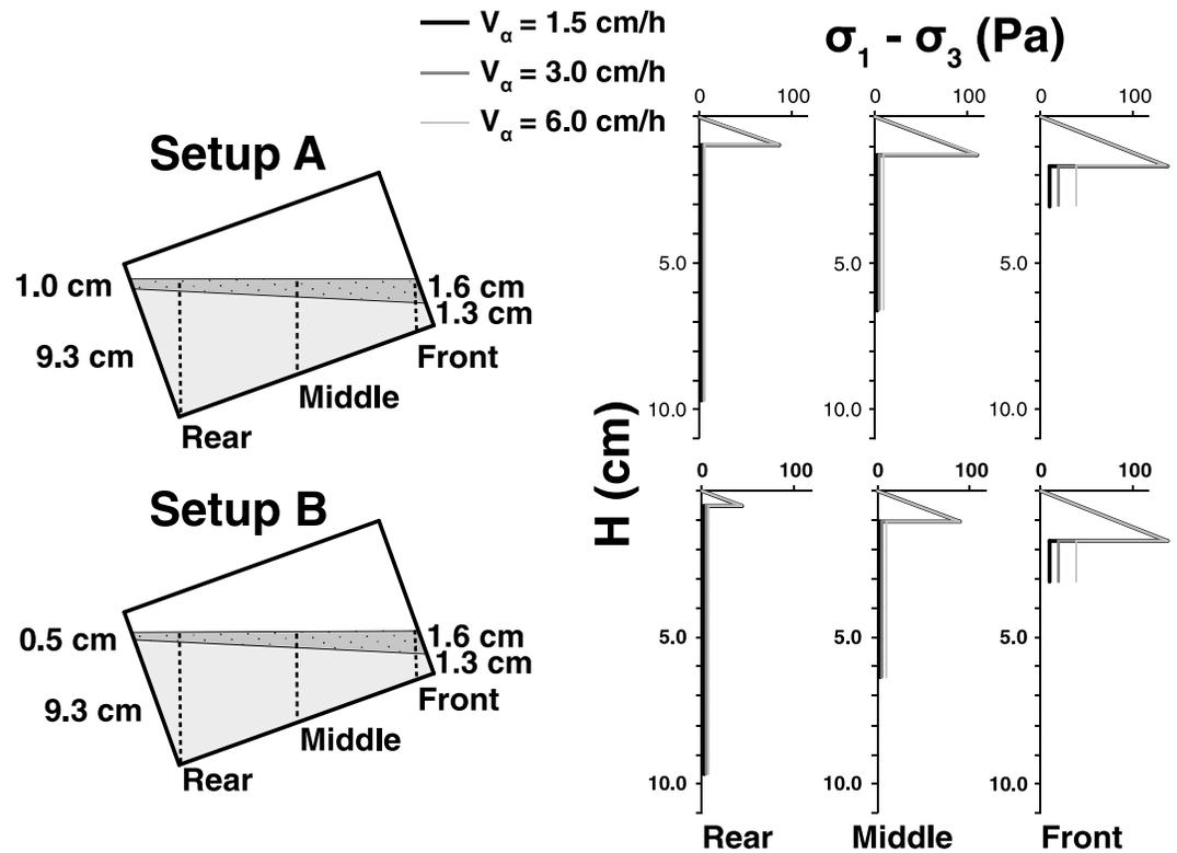
**Figure 6.** Model's side view and calculated strength profiles along a central transect for the two different initial geometries used in the experiments (reflecting the thickness variation in the frictional layer). Due to the variation of the sand layer thickness and displacement velocity, different strength profiles are calculated for the frontal (near the rotating wall), the middle, and the rear part (near the backstop) of the model.
