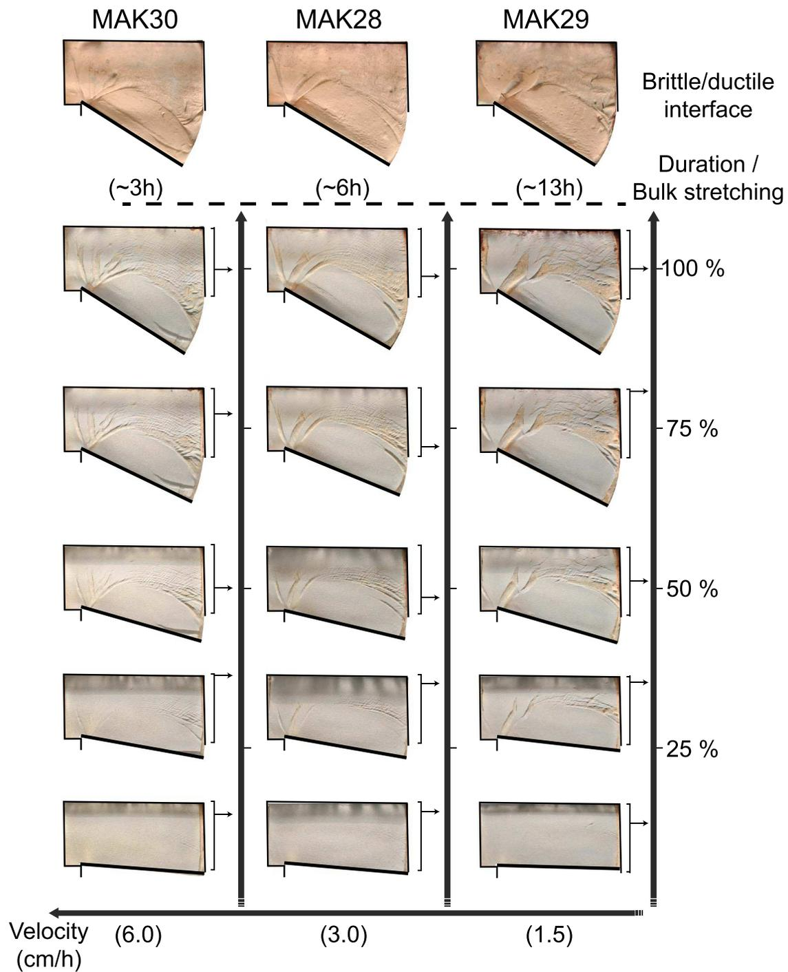
**Figure 9.** Selected top-view snapshots for Setup B experiments (thinner sand layer; see Figure 6) using three tested displacement velocities. The brittle-ductile interface at the end of each experiment is also shown at the top. To facilitate the discussion, a virtual north is taken as facing upward. See text for details.
