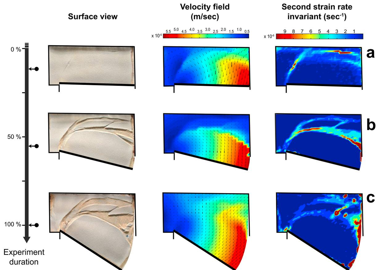
**Figure 11.** Selected top-view snapshots and calculated velocity field and second strain rate invariant of experiment MAK27 approximately at the (a) beginning, (b) midway, and at (c) the end of the experiment. The PIV calculations were made using PIVlab v.1.35 software (<http://pivlab.blogspot.gr/>). The curve-shaped pattern of the velocity field is typical for rotational driven deformation with the displacement magnitude reducing toward the pivot point. See text for details.
