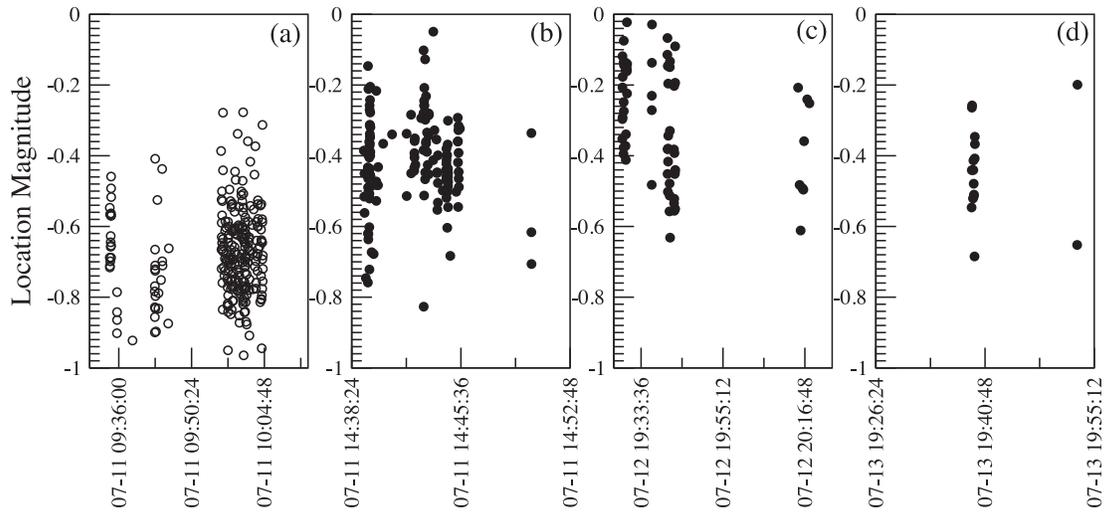
**Figure 8.** (a) Location magnitude of acoustic events associated to the excavation activity (250 events). (b) Location magnitude of the burst of acoustic events recorded on July 11 (191 events). (c) and (d) Location magnitude of the microseismic events recorded on July 12 (71 MSEs) and 13 (16 MSEs), respectively.
