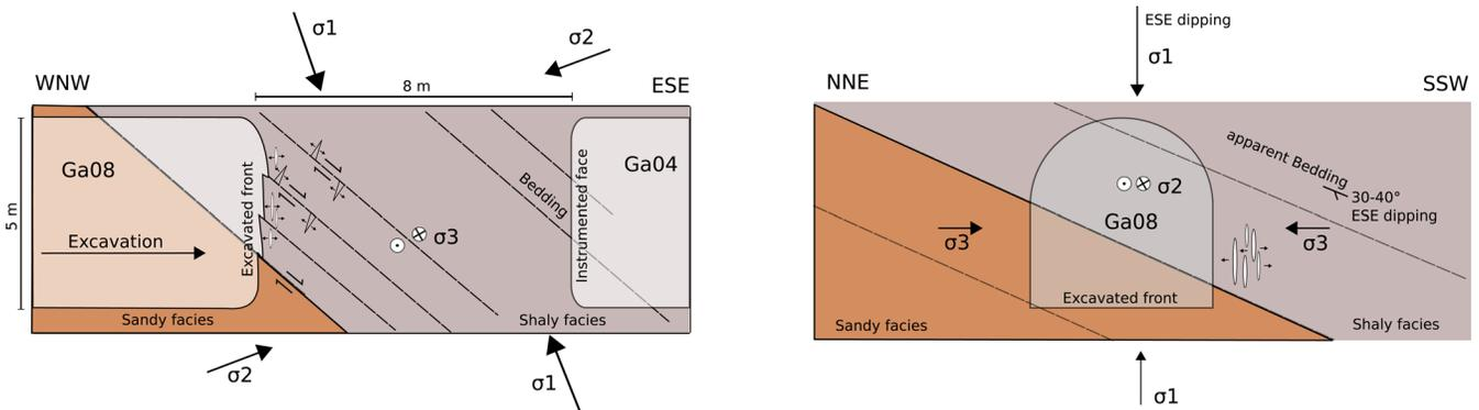
**Figure 11.** Conceptual representation of the stress pattern around an underground gallery excavated in a rock formation where the undisturbed maximum principal stress  $\sigma_1$  is subvertical and compressive: (a) Side view from shaly facies sidewall (modified from Nussbaum *et al.* 2011) and (b) View from Ga08 in the direction of the excavation front.
