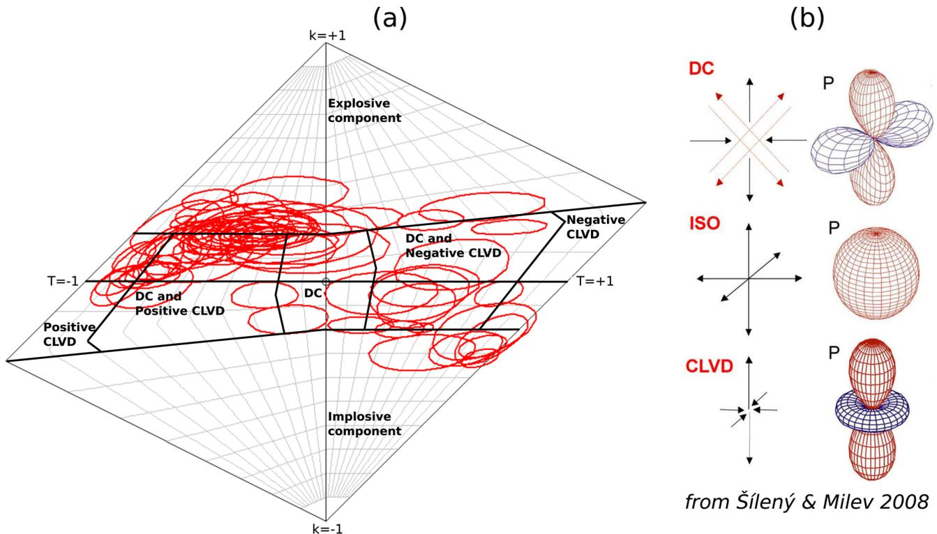
**Figure 9.** (a) Source mechanisms of the fully processed waveforms of 61 MSEs plotted in a Hudson  $T$ - $k$  plot with the red error ellipses related to the Moment Tensor inversion accuracy (average amplitude residual and standard deviation of the inversion operation: 0.13 and 0.07, respectively). The bold lines delimit the areas defined by Forney (1999). (b) Illustrations of the ISO, DC and CLVD mechanisms (modified from Šílený & Milev 2008).
