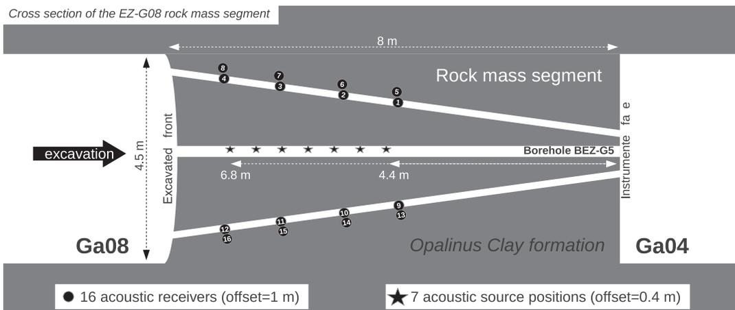
**Figure 2.** Schematic cross section of the rock mass segment (after 2008 July 12, 6 p.m.). The excavation operation comes from the left-hand side (gallery Ga08) and the opposite face (gallery Ga04) was instrumented for acoustic measurements. Ultrasonic measurements involve an active source that was introduced at different depths (black stars) in a central borehole (BEZ-G5). Sixteen acoustic receivers (black points) composed the acoustic arrays introduced in subhorizontal boreholes.
