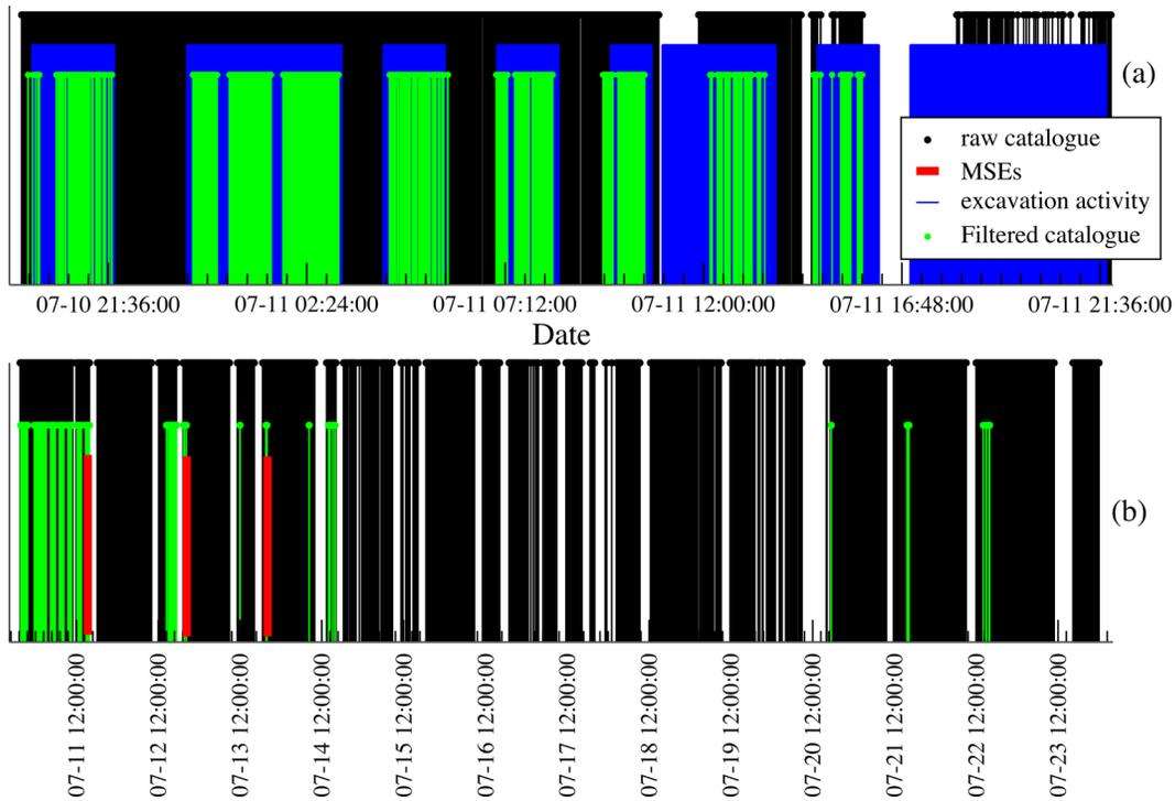
**Figure 3.** Time history of the 56 446 events of the raw data set (black lines) detailed for the period of excavation activity before July 12 (a) and for the whole period of experiment between July 10 and 23 (b). After the multistep filtering method, 20 per cent of the events are kept (green lines), in coherence with the time schedule of the excavation operation (blue zones). Finally, only 278 MSEs have been identified, located at three main time periods (red lines).
