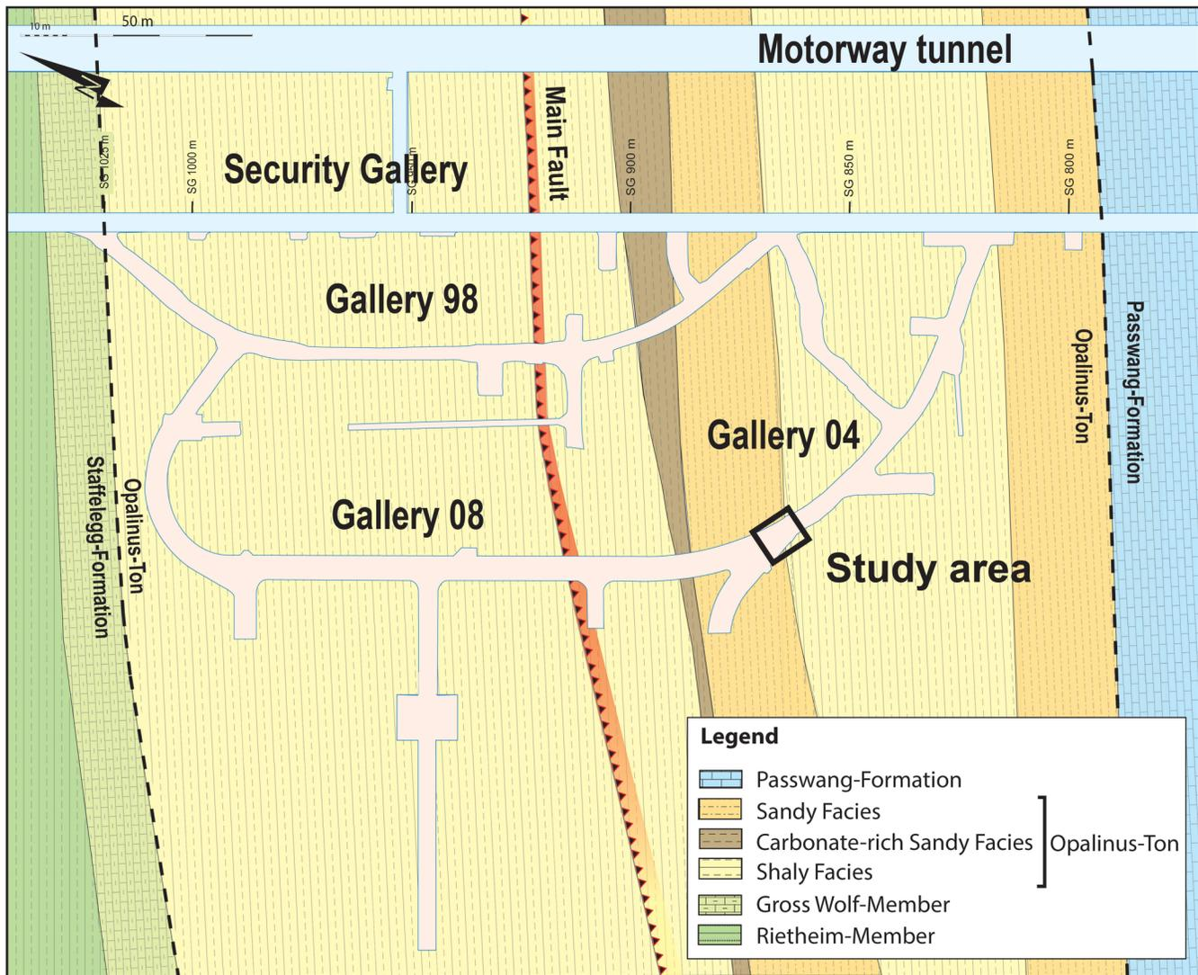
**Figure 1.** General view of geological map of the Mont Terri URL. The black box indicates the location of the so-called EZ-G08 experiments, at the junction between galleries Ga08 and Ga04 with the north and south sidewalls in a sandy and shaly facies, respectively.
