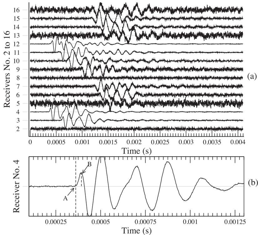
**Figure 5.** (a) Illustration of the 15 raw waveforms of an event belonging to the MSE catalogue (normalized amplitudes). (b) Details of the waveform recorded on channel No. 4: the arrows A and B point towards the arrival time and amplitude of the first movement, respectively.
