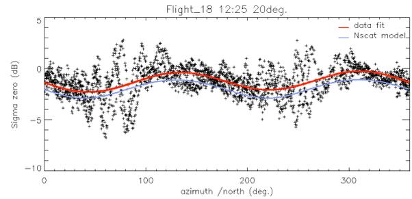
Fig. 5. Normalized radar cross-section at incidence  $20^\circ$  as a function of azimuth for the same conditions as the red line in Fig.4. Here the red line is a fit (Fourier development with 2 harmonics), the blue line the NSCAT model [9] for the same wind conditions ( $9 \text{ m s}^{-1}$ ).
