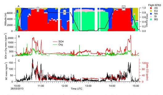
Figure 4. (a) The flight altitude and FLEXPART FPES fractions for each source region during B763, the plume locations during SLR are marked as i, ii and iii and grey lines along the flight altitude track; (b) the time series of organic matter and sulphate; (c) BC mass and CO concentration.
