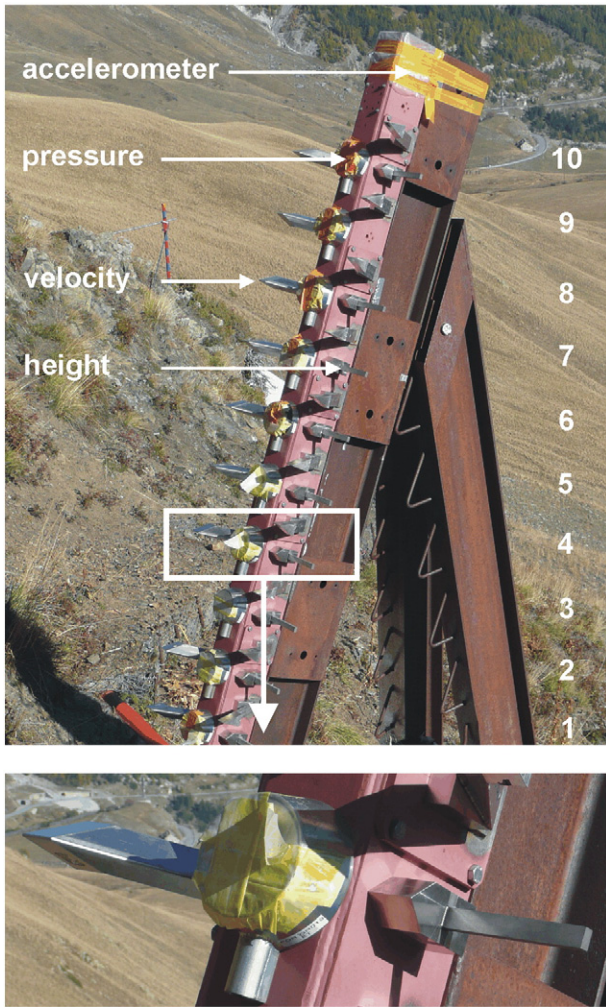
Fig. 5. Top: Steel tripod set up in avalanche path no. 2 and supporting velocity, pressure and height sensors to record the vertical profile within the avalanche. An accelerometer is fixed inside at the top (not visible) to measure the structure displacement for a check on the boundary conditions of the pressure sensors. Numbers refer to pressure measurements plotted in Fig. 6. Bottom: Zoom on the 3 sensors recording at a given flow depth.
