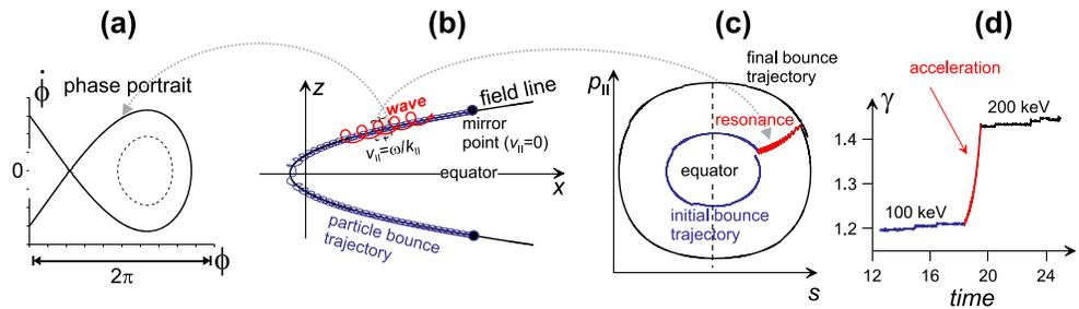
**Figure 1.** (a) Phase portrait of system (2) for  $A < B$ . (b) Schematic view of the system. (c) Particle trajectory in  $(s, \rho_{\parallel})$  space. Black and blue colors are used for final and initial bounce oscillations, while red color shows trapped particle motion. (d) Particle gamma factor as a function of time.
