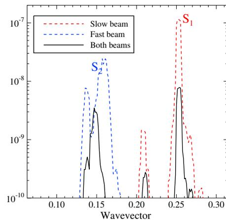
**Figure 12.** Comparison of the density fluctuation spectra showing the level of generated ion acoustic waves at time  $\omega_{pe}t = 1.5 \times 10^4$  when the slow beam only (in dashed red), the fast beam only (in dashed blue), or both beams (in full black) are considered.
