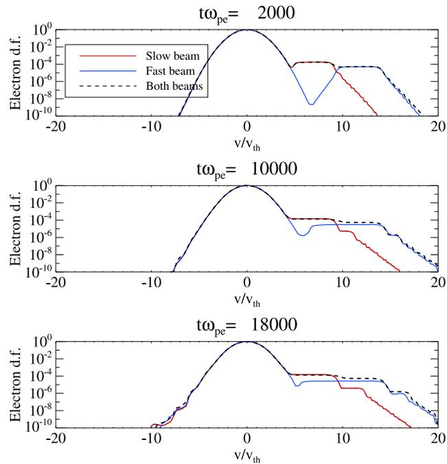
**Figure 11.** Comparison of the velocity electron distribution functions, averaged on the numerical box, at (from top to bottom) three successive times  $\omega_{pe}t = 2 \times 10^3$ ,  $10 \times 10^3$  and  $18 \times 10^3$ , when the slow beam only (in full red), the fast beam only (in full blue), or both beams (in black dashed) are considered.
