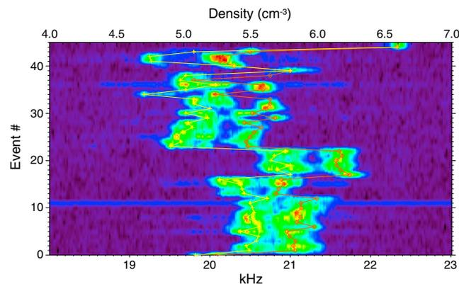
**Figure 6.** Spectrum around the plasma frequency for all the events of the compact group. The ordinate axis displays the event number, an indication of time (but the events are not regularly observed in time). The red (yellow) line displays the location of the upper (lower) Langmuir peak. The upper abscissa scales the electron density corresponding to the frequencies of the lower axis.
