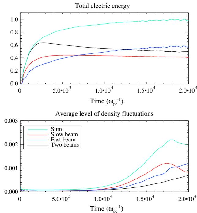
**Figure 9.** Evolution of the (top) total electric energy and (bottom) average level of density fluctuations when the slow beam only (red), the fast beam only (blue), or both beams (black) are present. The green line shows the sum of the isolated contribution of the two beams. To ease the reading, the electric energy is normalized to the maximum of electric energy corresponding to the sum of the electric energy when the beam is isolated.
