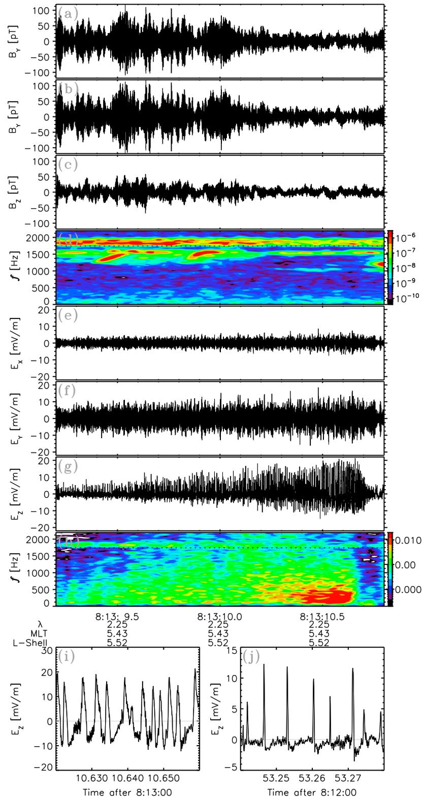
**Figure 1.** Three components of the (a–c) magnetic and (e–g) electric field perturbations in magnetic-field-aligned coordinates measured on Van Allen Probes B on 1 November 2012. Dynamic spectra of the (d) perpendicular magnetic and (h) parallel electric fields are shown (black dot lines indicate  $0.5f_{ce}$ ). (i and j) More detailed  $E_z$  waveforms.
