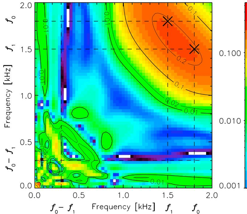
**Figure 3.** The bicoherence spectrum of the two transverse magnetic field components and the parallel component of the electric field. Dashed lines indicate frequencies of observed whistler waves ( $f_0$  and  $f_1$ ) and the frequency of EAW ( $f_0 - f_1$ ). Crosses indicate the supposed positions of peaks on cross-frequencies ( $[f_0, f_1]$  and  $[f_1, f_2]$ ) in a case of their phase connection.
