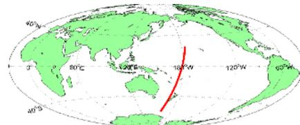
**Figure 3. Orbit track when CALIPSO spacecraft is tilted 30° backward on July 17, 2014.**
