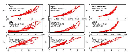
**Figure 2.** Scatter plot of the DC component of the thermospheric density versus the DC component of various solar inputs. The RMS and Spearman's correlation coefficient *r*, together with their standard deviation, are indicated for each proxy. The standard deviation has been obtained by bootstrapping. In all plots, a linear model  $\hat{\rho}_{DC} = \alpha + \beta x_{DC}$  is used for computing the RMS. Densities are in units of  $[10^{-14} \text{ kg m}^{-3}]$ .)
