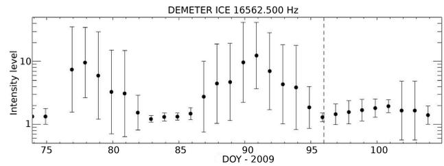
**Fig. 2.** Variation of the DEMETER observed signal at the frequency of 16 652.5 Hz (the closest frequency to the German transmitter signal 16 560 Hz) versus the day of the year 2009 (from 15 March to 11 April 2009). The day of the EQs is indicated by a vertical dashed line.
