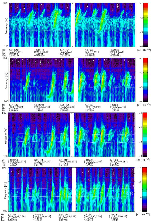
**Fig. 1.** Detailed time-frequency power spectrograms of magnetic field fluctuations near the source region captured by the SCM instruments onboard four THEMIS spacecraft on 17 July 2007. Panels (from top to bottom) show data from THB, THC, THD, and THE, respectively. Magnetic dipole latitude, magnetic shell, and SM coordinates are given for all s/c. Radial distances are from 10.6 to 11.5  $R_E$ , and MLT is about 13:30 UT during this interval.
