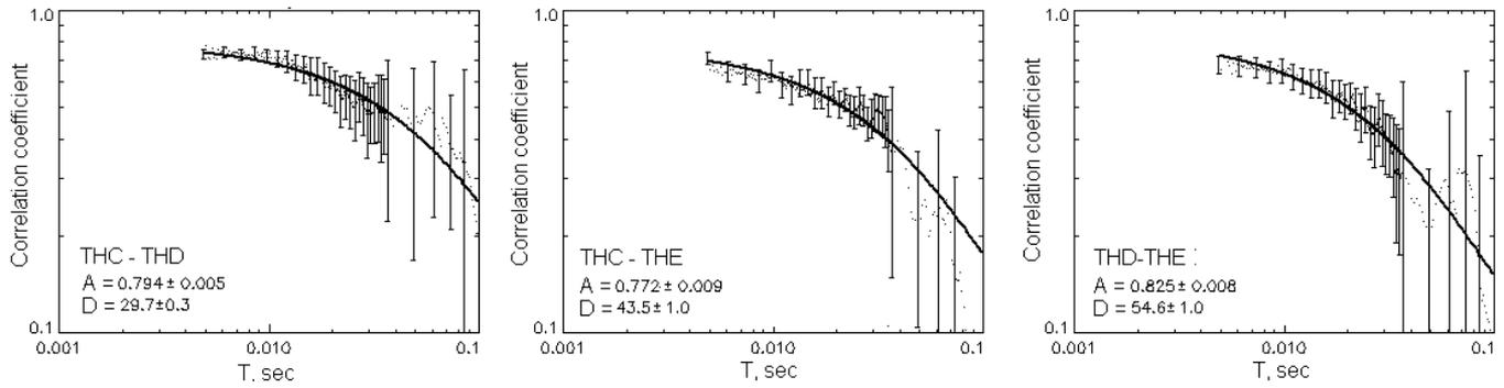
**Fig. 4.** Cross-correlation analysis of the discrete chorus element observed at 13:12 UT on 17 July 2007 onboard THEMIS spacecraft. The correlation coefficient time dependence is shown for spacecraft THC-THD, THC-THE, and THD-THE, respectively. The approximation with  $\frac{(1-e^x)}{x}$  function is shown with solid line. The approximation parameters are listed.
