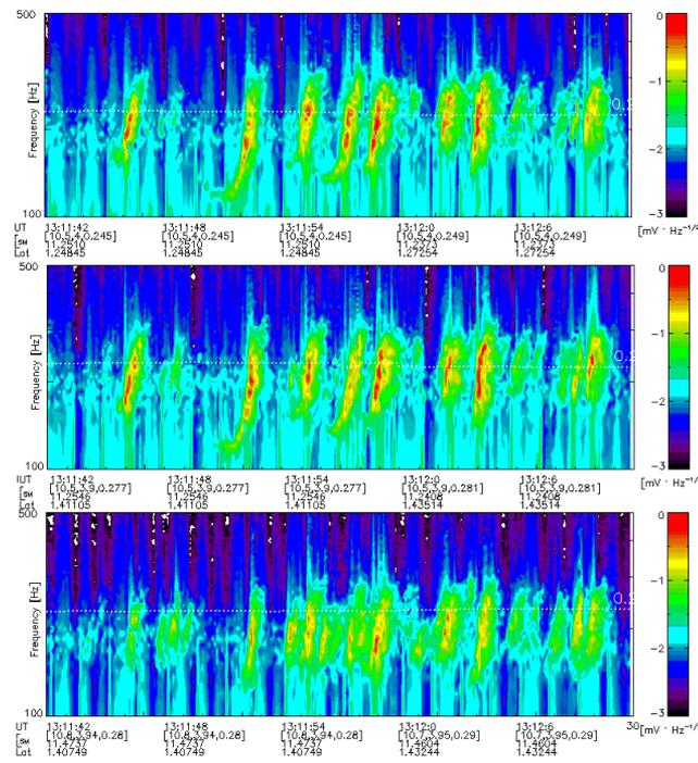
**Fig. 2.** Detailed time-frequency power spectrograms of electric field fluctuations near the source region captured by the EFI instruments onboard four THEMIS spacecraft on 17 July 2007. Panels (from top to bottom) show data from THC, THD, and THE, respectively. Magnetic dipole latitude, magnetic shell, and SM coordinates are given for all s/c. Radial distances are from 10.6 to 11.5  $R_E$ , and magnetic local time is about 13:30 UT.
