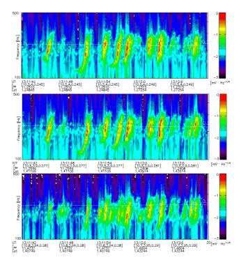
**Fig. 2.** Detailed time-frequency power spectrograms of electric field fluctuations near the source region captured by the EFI instruments onboard four THEMIS spacecraft on 17 July 2007. Panels (from top to bottom) show data from THC, THD, and THE, respectively. Magnetic dipole latitude, magnetic shell, and SM coordinates are given for all s/c. Radial distances are from 10.6 to 11.5  $R_{\rm E}$ , and magnetic local time is about 13:30 UT.
