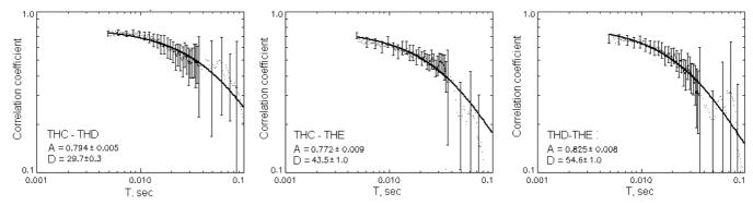
**Fig. 4.** Cross-correlation analysis of the discrete chorus element observed at 13:12 UT on 17 July 2007 onboard THEMIS spacecraft. The correlation coefficient time dependence is shown for spacecraft THC-THD, THC-THE, and THD-THE, respectively. The approximation with  $\frac{(1-e^x)}{x}$  function is shown with solid line. The approximation parameters are listed.
