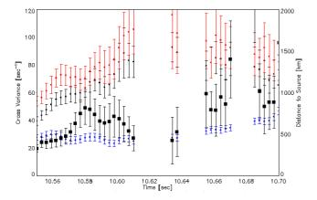
**Fig. 5.** The time dynamics of variation coefficients  $D_{\rm Sij}$  obtained from waveforms of the THC, THD, THE spacecraft is shown with black, blue and red circles (amplitude is marked on the left scale). The time dynamic of distance from THC spacecraft to the source region is shown with black squares (amplitude is marked on the right scale).
