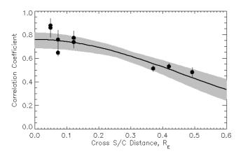
**Fig. 6.** The amplitude level correlation coefficients of the SCM magnetic field and EFI electric field waveform captured onboard THEMIS spacecraft at 13:12 UT on 17 July 2007 in dependence on cross spacecraft distances.
