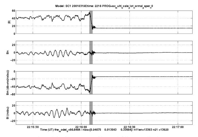
**Figure 1.** The magnitude and three components of the magnetic field as measured by Cluster 1 magnetometer on 19.03.2001 during the crossing of the terrestrial bow shock.
