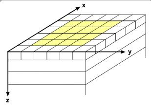
**Fig. 1** Heterogeneous thin-sheet model at the surface, with normal (*white*) and anomalous (*yellow*) conductance embedded in a layered (1D) host medium. The resistivities and thicknesses of the 1D host medium are held fixed and determined from *a priori* information
