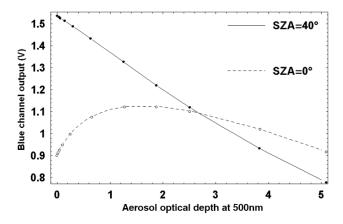
**Figure 1.** Solar flux received by ODS in the blue wavelength range as a function of the aerosol optical depth (AOD), at 40° SZA (solid line with black circles) for total direct and scattered sunlight and at 0° SZA (dashed line with white circles) for scattered sunlight only. The ratio between the two fluxes varies monotonously, with AOD providing a direct AOD measurement independent of sensor calibration.
