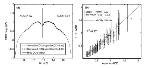
**Figure 15.** (a) Evolution of ODS signal measured on 5 January 2005 and those simulated for the AOD values obtained by the retrieval procedure of dust opacity using only half of the day. (b) Correlation between ODS blue channel and AERONET AOD at 370 nm for cloud-free days, and where two values of AOD per day have been estimated for days with a daily average AOD above 0.8.
