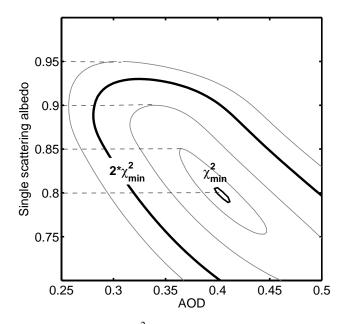
**Figure 16.** Contours of  $\chi^2$  in the AOD- $\omega$  space for the ODS test signal. The minimum of  $\chi^2$  is found for AOD = 0.4 and  $\omega$  = 0.8.
