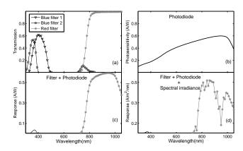
**Figure 3.** (a) Blue- and red-filter transmission. (b) Photodiode spectral response. (c) Response of filters—photodiodes combination. (d) Final blue-channel response  $(370 \, \mu m \pm 20 \, \mu m)$  on the left and red-channel response  $(902 \, \mu m \pm 169 \, \mu m)$  on the right.
