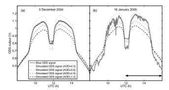
**Figure 8.** Comparison between ODS blue channel observed output voltage and simulated blue ODS signal for AOD values of 0.1, 0.6 and 1 (a) in cloud-free conditions on 5 December 2004 and (b) on 16 January 2005 in cloudy conditions.
