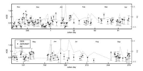
**Figure 13.** AOD derived from ODS blue channel (grey dots with error bars) and AERONET (squares) at 370 nm between November 2004 and October 2005. The grey dashed line represents the relative error that is defined in Eq. (4).
