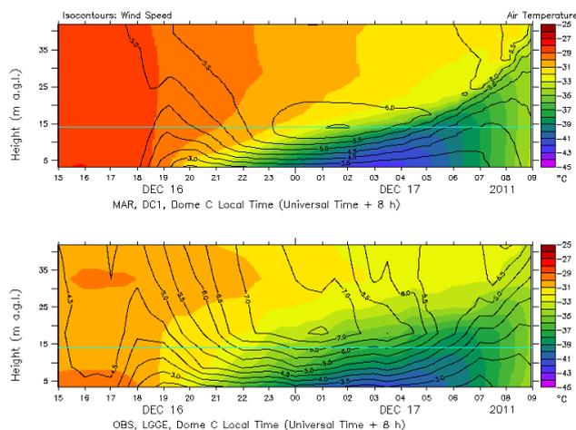
**Figure 2.** Temperature (colour) and wind speed (isocontours) at the Dome C tower, simulated by MAR on 16–17 December 2011 (upper panel) and observed (lower panel). Local Time LT (Universal Time UT + 8 h) is used. The simulated jet level is at  $z = 14$  m a.g.l. (shown by a cyan line in both panels).
