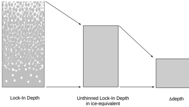
**Figure 2.** Scheme of different representations of a firm column. (Left) When the firm column is at surface, its height is equal to the lock-in depth. (Middle) If one virtually converts the firm column into cumulated ice-equivalent accumulations, one gets the unthinned lock-in depth in ice equivalent (ULIDIE). (Right) When the firm column is buried down into the ice sheet and encounters vertical thinning, its height decreases to  $\Delta$ depth.
