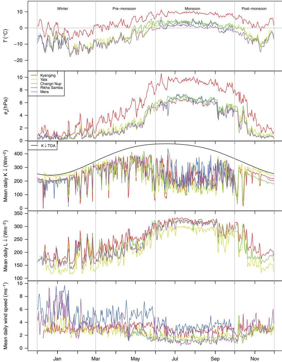
Figure 2. Summary of mean daily 2012–2013 meteorological data. From top to bottom, air temperature ( $T$ ), vapour pressure ( $e$ ), incoming short-wave radiation ( $K \downarrow$ ), incoming long-wave radiation ( $L \downarrow$ ), and wind speed ( $u$ ). Climatological seasons (see text) are shown as vertical grey lines, and extraterrestrial global radiation calculated for 28N, 85E is given in black.
