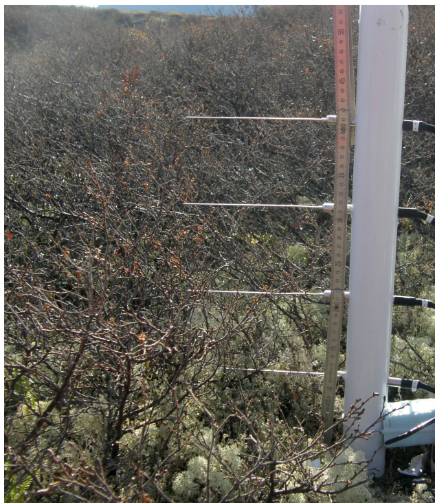
Figure 1. Photograph of the four TP02 needle probes deployed in shrub tundra. The photo was taken on 6 October 2014, when the dwarf birch had grown to about 30 cm high. The needle probes are 14, 24, 34 and 44 cm above the ground–lichen interface.
