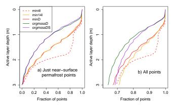
**Figure 9.** The vertical distribution of permafrost, shown by the fraction of points for which the soil thaws below a given depth. (a) Nearsurface permafrost points only: this includes only those points with ALT less than 3 m, and hence 0 % of them thaw to below 3 m. (b) All points are included, so about 70 % thaw to greater than 3 m or have no permafrost at all. There is one point for each grid cell for each year of the historical simulation.
