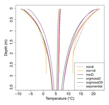
**Figure 10.** The annual maximum, minimum and mean of simulated soil temperatures (right-hand, left-hand and centre lines respectively), averaged over the period 1979–1989, for the land area north of  $50^{\circ}$  latitude. Comparing the simulations with different soil depth is of particular interest here.
