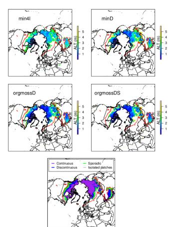
**Figure 7.** First two rows: mean active layer thickness in JULES simulations, 1979–1989. All grid cells with active layer  $\leq 6$  m are shown, with mean ALT indicated by colour. Bottom: observed permafrost map (Brown et al., 1998), based on maps made between approximately 1960 and 1990. On all plots the 0° air temperature isotherm is shown in red (1979–1989 from WFDEI air temperature, see Sect. 2.4.1).
