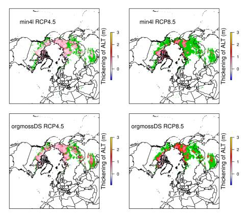
**Figure 12.** Coloured area shows near-surface permafrost at the start of the simulation: green regions have disappeared by the end of the simulation (2090–2100) and other colours (reddish) show active layer deepening in the remaining permafrost.
