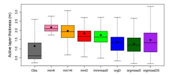
**Figure 4.** Simulated and observed range of active layer depths for CALM sites (Sect. 2.4.3). Black dots are means, the boxes shows the interquartile range (IQR) and the horizontal line is the median. The whiskers indicate the most extreme data point that is no more than 1.5 times the IQR. Outliers are not shown. Points at which either the simulated or observed active layer was very large (greater than 6 m) were removed. The model point for each CALM site is the grid box containing that site.
