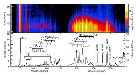
Figure 1. (top) The IUVS's FUV and MUV detectors color composite generated using a full vertical scan from orbit 110 (2059 UTC, 18 October 2014), one of the 744 profiles. The horizontal and vertical axes represent wavelength and altitude (80 – 250 km), respectively. (bottom) Calibrated FUV and MUV spectra obtained from the same scan; these are averages of 13 individual spectra obtained between 120 and 135 km.
