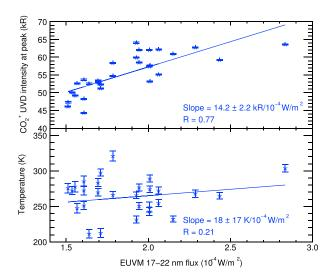
**Figure 5.** Short-term variations of (top)  $CO_2^+$  doublet maximum intensity and (bottom) topside temperature with 17–22 nm irradiance measured by the EUVM instrument aboard MAVEN. Values are for  $L_S \sim 337-343^\circ$  (orbits 1160–1220) and SZA between 30° and 40°. R is the linear correlation coefficient.
