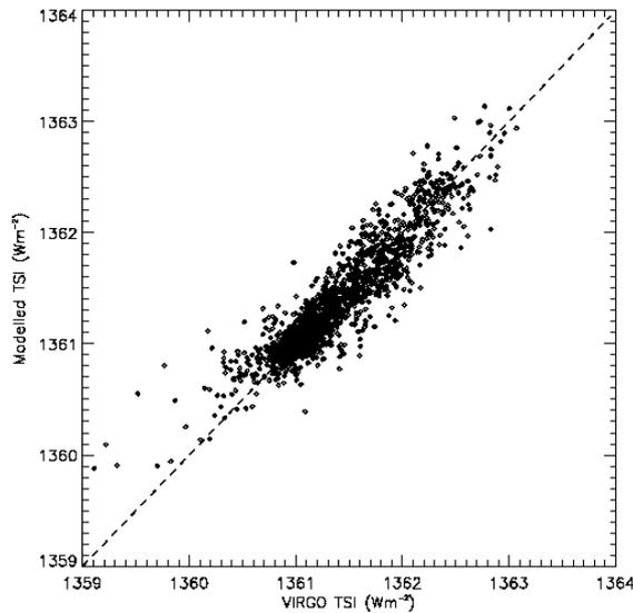
**Fig. 19.** Scatter plot between the VIRGO TSI data and the fitted data based on our regression analysis. The squared correlation coefficients of the fit versus the VIRGO observation is  $r^2 = 0.88$ . The dashed line indicates equality between the two data sets.
