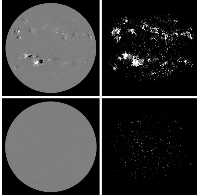
**Fig. 11.** Left panel: magnetograms from the solar maximum (top left) and solar minimum (bottom left). Right panel: magnetic region segmentation maps from solar maximum (top right) and solar minimum (bottom right). The negative and positive regions on the magnetogram images are represented as grey and white regions respectively on the segmentation map, for clarity purpose.
