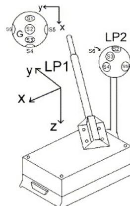
FIG. 1. Segmented Langmuir probe (left) and illustration of the various segments (right). Reprinted with permission from Lebreton *et al.*, Planet. Space Sci. **54**, 472 (2006). Copyright 2006 Elsevier.
