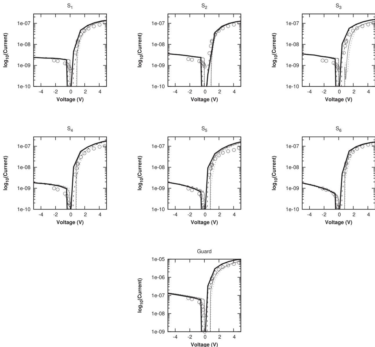
FIG. 3. Comparison between the simulated and measured I-V curves for segments  $S_1, S_2, S_3, S_4, S_5, S_6$  and the guard electrode. The thicker lines show the characteristics for the fast scan and thinner lines show the characteristics for the slow scan. In both cases, the solid lines are for the up scan (negative to positive) and dashed lines for the down scan (positive to negative). Circles show the characteristics obtained from the reference case.
