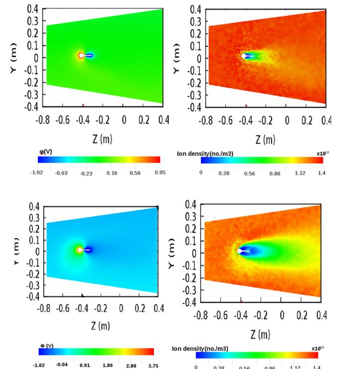
FIG. 2. Profiles of the sheath potential (left) and the corresponding wake in ion density behind the probe (right). Plasma is drifting in the Z direction, whereas the orbital velocity of the satellite is in the  $-Z$  direction.
