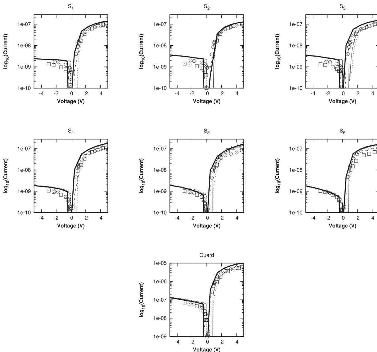
FIG. 4. Comparison between the measured and simulated I-V curve of segments  $S_1, S_2, S_3, S_4, S_5, S_6$  and the guard electrode, showing the effect of the ion composition. The measured characteristics and the reference case are the same as in Figure 3. Circles represent the characteristics obtained with the reference case and squares show the characteristics computed with 100%  $O^+$  ions.
