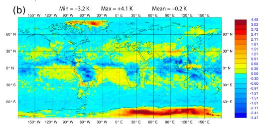
Figure 2. First-guess departures (observed BTs – those calculated from the forecast background) for Suomi-NPP/ATMS (a) channel 18  $(183 \pm 7 \, \text{GHz})$  and (b) channel 22  $(183 \pm 1 \, \text{GHz})$  and the current ECMWF NWP system. The maps show the mean, with the global minima, maxima and means in the legend.
