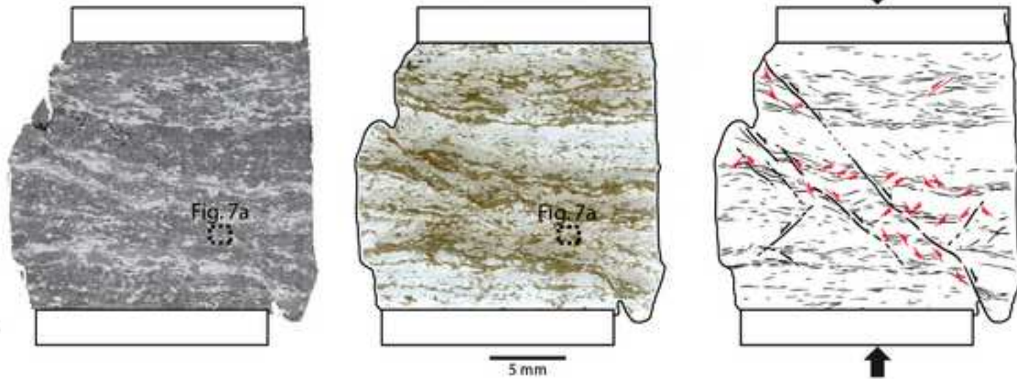
b) He/900/21-32: \dot{\gamma}=10^{-4}-10^{-3} \text{ s}^{-1} , Strain=27%, Glass=21±7 - 32±6%
