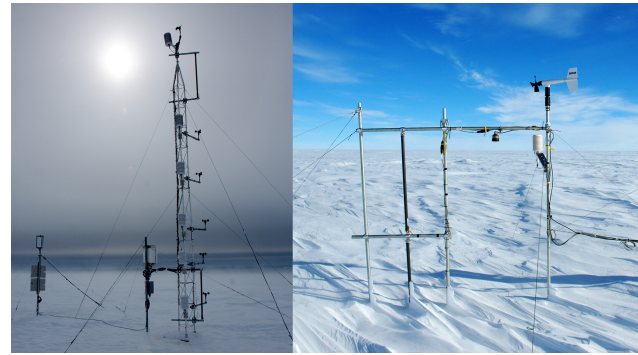
Figure 2. Left: the D17 7 m mast with one second-generation FlowCapt™ sensor. Right: the D47 automatic weather and snow station with two second-generation FlowCapt™ sensors.
