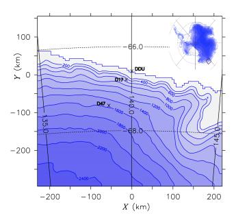
**Figure 1.** Integrative domain of the MAR in Adélie Land, East Antarctica. The crosses mark the location of the French Dumont d'Urville base (DDU) and the two automatic weather and snow stations used in this study (D17 and D47).
