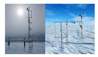
**Figure 2.** Left: the D17 7 m mast with one second-generation FlowCapt<sup>TM</sup> sensor. Right: the D47 automatic weather and snow station with two second-generation FlowCapt<sup>TM</sup> sensors.
