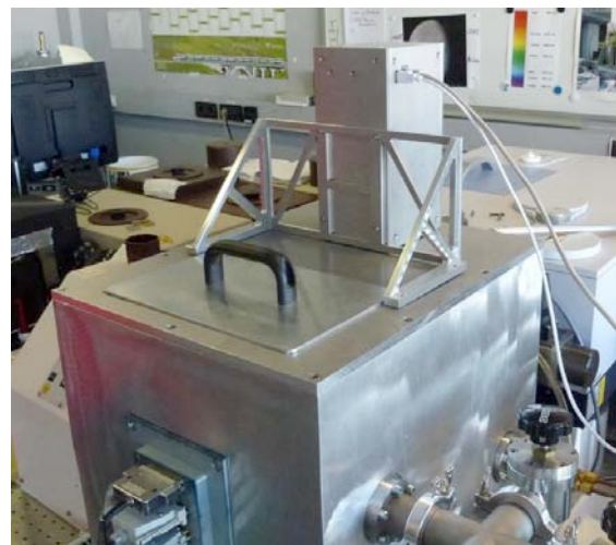
Figure 4. VEM breadboard on the high temperature chamber at PEL [9,10].
