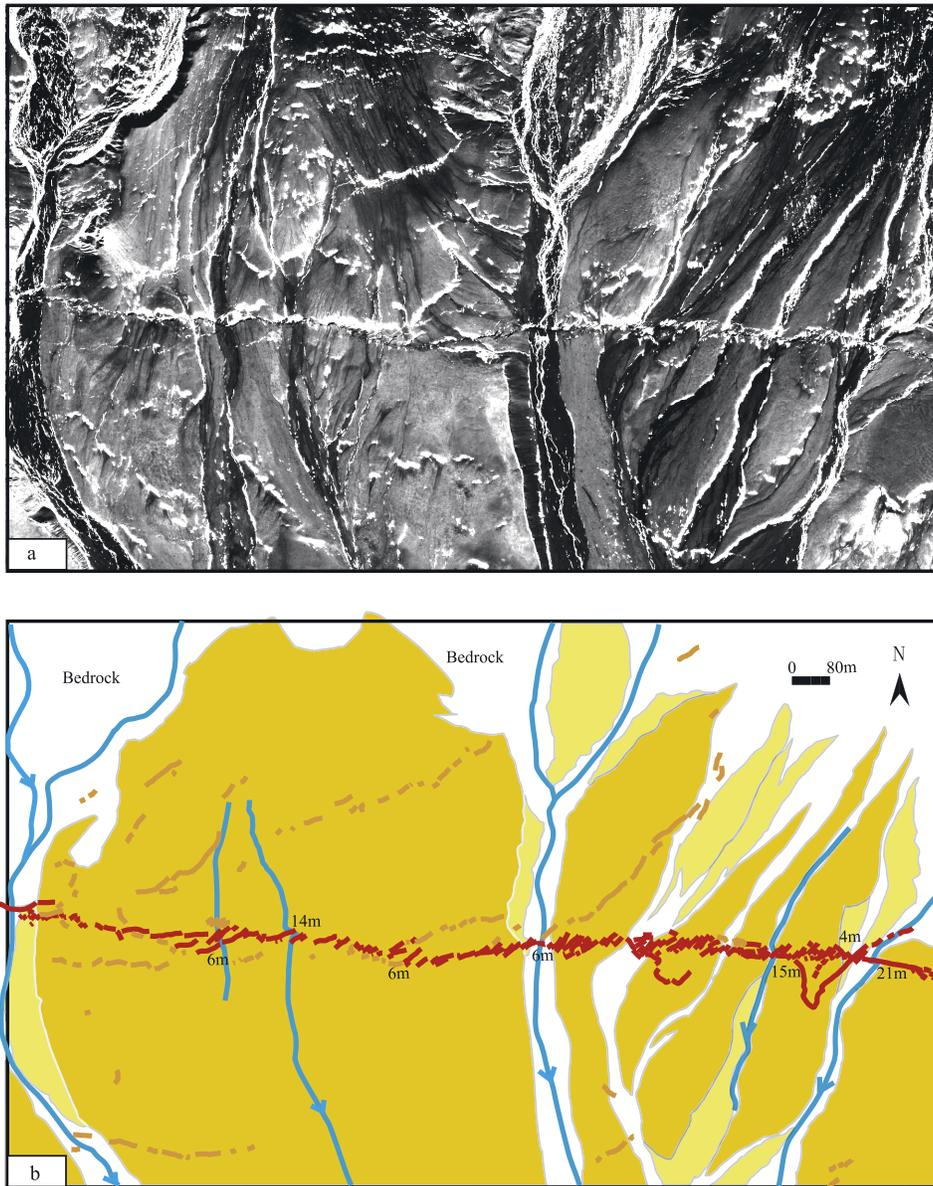
**Figure 16.** (a) Ikonos image created on 6 January 2003 that covers the area where *Lin et al.* [2002] gave a coseismic horizontal displacement of about 13.5 m. (b) Detailed strip map showing the surface rupture pattern of the Kunlunshan earthquake and coseismic horizontal displacements on different rupture strands. The legends are same as Figure 15.
