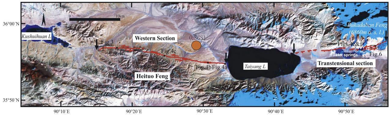
**Figure 2.** Map showing the surface breaks of the 2001 Kunlunshan earthquake on the western and transtensional sections based on field observations and high-resolution satellite images. Black arrows indicate the terminal point of the surface breaks of the different sections. Blue triangles are hot springs.
