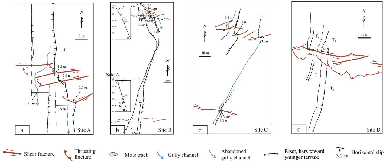
**Figure 13.** Measured topographic map showing surface rupture pattern and coseismic left-lateral and vertical displacements on the Yuxi Feng subsection (locations are marked in Figures 1b and 11). (a) Site A ( $35.767^{\circ}\text{N}$ ,  $93.323^{\circ}\text{E}$ ). (b) Site B ( $35.767^{\circ}\text{N}$ ,  $93.325^{\circ}\text{E}$ ). (c) Site C ( $35.762^{\circ}\text{N}$ ,  $93.398^{\circ}\text{E}$ ). (d) Site D ( $35.814^{\circ}\text{N}$ ,  $92.955^{\circ}\text{E}$ ).
