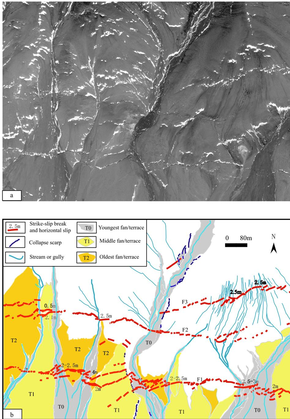
**Figure 15.** (a) Ikonos image created on 6 January 2003, around the site  $93.365^{\circ}\text{E}$  where *Lin et al.* [2002] gave a maximum coseismic horizontal displacement of 16.3 m. (b) Detailed strip map showing the surface rupture pattern of the Kunlunshan earthquake and coseismic horizontal displacements on different rupture strands. Blank areas are the pre-Quaternary of Kunlun Range.
