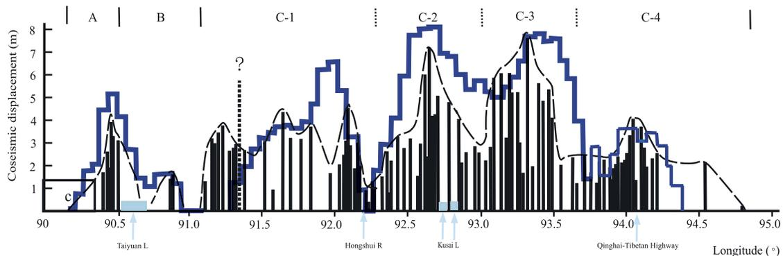
**Figure 14.** Distribution of the measured horizontal coseismic horizontal displacements along the strike of the surface rupture zone. Blue lines represent the coseismic horizontal displacements inferred from INSAR data [Lasserre et al., 2005]. Other legends are the same as in Figure 1. Horizontal displacements are collected from Xu et al. [2002b], Dang and Wang [2002], Chen et al. [2003], and also measurements in the field.
