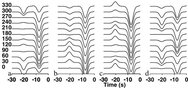
**Figure 4.** Synthetic P components for deformed wadsleyite: (a) shear in the vertical direction, shear plane is in the azimuth of  $90^\circ$ ; (b) horizontal shear plane, azimuth of shear is  $90^\circ$ ; (c) horizontal foliation plane, azimuth of lineation is  $0^\circ$ ; (d) vertical foliation plane in the azimuth of  $0^\circ$ , lineation is vertical. Origin of the time axis is arbitrary. Numbers attached to the traces are back azimuths in degrees.
