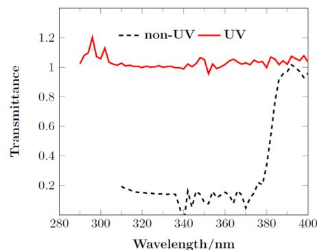
**Figure 1.** Transmittance as measured for the control and the UV plates. The UV plate transmits solar UV above 290 nm, whereas the control plate has a cutoff at ca. 375 nm (note that the control plate has an average transmittance of 15 % below 375 nm). As transmission was measured as the ratio between solar light below plexiglass plate to light above the plexiglass plate, light reflected back by the snow might lead to transmittance greater than 1.
