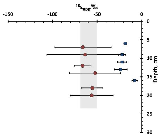
**Figure 11.** The depth profile of  $^{15}\epsilon$  for the UV pit. The  $^{15}\epsilon$  was calculated from samples collected at the same depth during each sampling event. Error bars are calculated using the least square fit method as in Frey et al. (2009). The shaded region represents the measured  $^{15}\epsilon$  range of  $-50$  to  $-70$  ‰.
