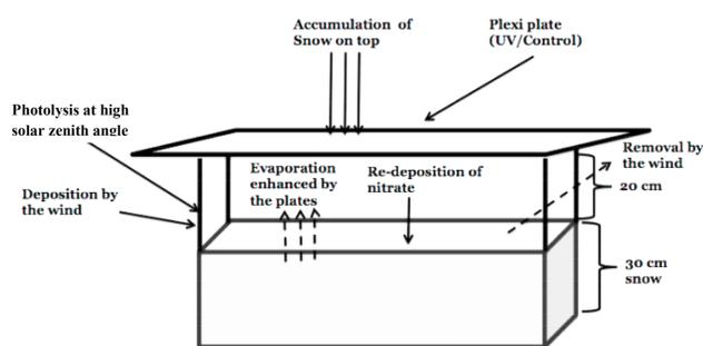
**Figure 9.** Schematic showing the possible external processes that could affect the surface layers of both the UV and control pits. These include evaporation, wind deposition and/or removal and photolysis at high solar zenith angle.
