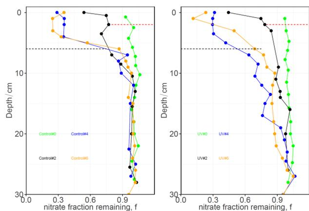
**Figure 3.** Plot of the nitrate fraction remaining in the snow ( $f$ ) with depth. Control samples (reduced solar UV) are plotted in the left panel and UV-exposed samples are plotted in the right panel. The numbers denote the sampling events, which were carried out at 10-day intervals from 2 December 2011 to 30 January 2012. The dashed lines show the depth where external factors (mainly mixing) play a significant role.
