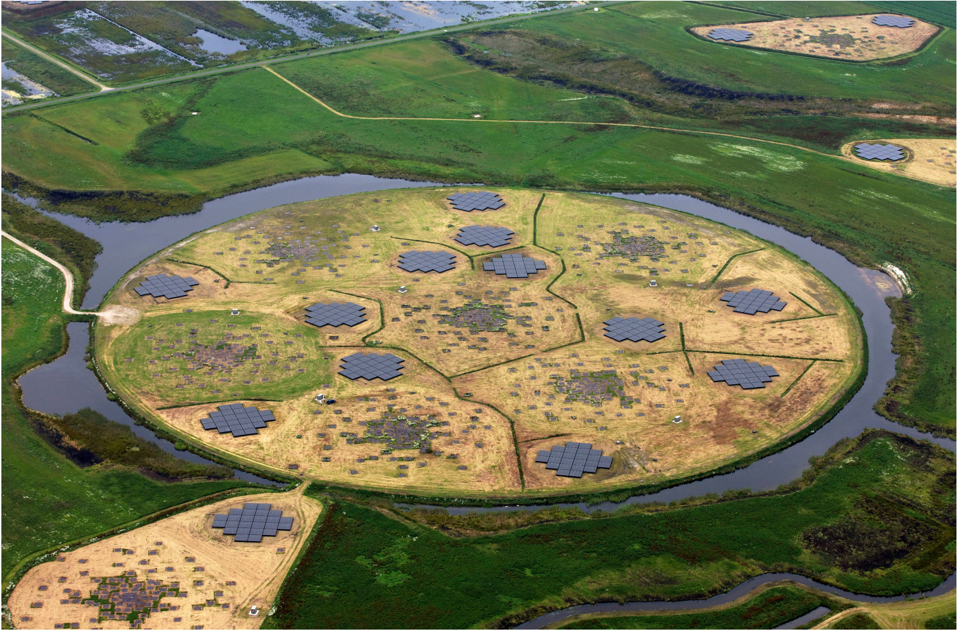
Fig. 1. Aerial photograph of the Superterp, the heart of the LOFAR core, from August 2011. The large circular island encompasses the six core stations that make up the Superterp. Three additional LOFAR core stations are visible in the upper right and lower left of the image. Each of these core stations includes a field of 96 low-band antennas and two sub-stations of 24 high-band antenna tiles each.
