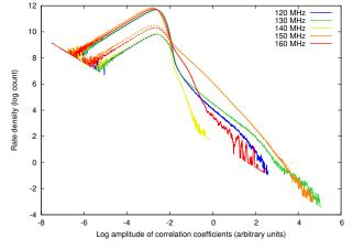
**Figure 8.** Histograms for 5 different 0.2 MHz HBA sub-bands without band-pass correction and flux calibration. The continuous lines represent the data before RFI flagging. The dashed lines are the histograms of the samples that have been classified as RFI.
