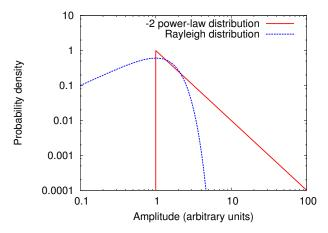
**Figure 3.** The Rayleigh and power-law distributions in a log-log plot. The power-law distribution (Eq. (5)) has a constant slope of -2 over the range it is defined. The slope of the Rayleigh distribution in the limit of the origin is 1. Its maximum occurs where the amplitude value equals its mode  $\sigma$ , which is 1 in this example. For higher amplitudes, its slope decreases exponentially.
