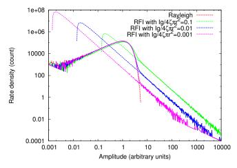
**Figure 4.** Histograms of simulated samples that all have a contribution of noise and RFI. Various settings of the parameters were used, and samples were drawn as described in Eq. (14). Solid lines: the combined distributions, dashed lines: the power-law distributions before mixing.
