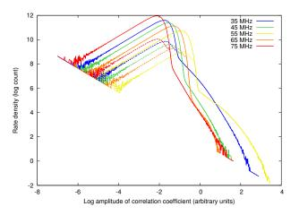
**Figure 7.** Histograms for 5 different 0.2 MHz LBA sub-bands without band-pass correction and flux calibration. The continuous lines represent the data before RFI flagging. The dashed lines are the histograms of the samples that have been classified as RFI.
