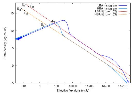
Figure 9. Observed LBA distribution after band-pass correction and flux calibration.  $S_{l1}$  and  $S_{l2}$  denote the limits of the distribution with a sharp lower cut-off (Eq. (18)) and uniform lower limit (Eq. (19)),  $S_d$  is the average lower limit of RFI that is detected.
