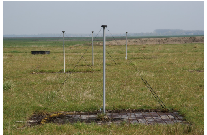
Fig. 2: Low-band antennas at the central core of LOFAR, the Superterp. In the background the black box of a LORA particle detector can be seen.
