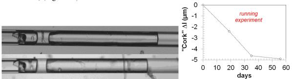
**Figure 2:** Left, capillary tube ( $\phi = 80 \ \mu m$ ) filled with NaCl brine and closed by two NaCl massive precipitates, with (upper,  $t_0$ ) and without (lower,  $t_0 + 56$  days) in-between dendritic solid. Right, decreasing size of the massive solids, showing the dissolution effect with time.
