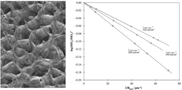
**Figure 3:** Silica paste pore network (left) in which (right) silica concentration (normalized to the initial concentration, symbols) is measured as a function of the extraction pressure, here converted into the corresponding pores sizes, and thermodynamic recalculation (lines).
