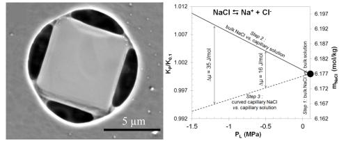
**Figure 1:** Left, normal and capillary halite precipitated in a pore initially saturated with aqueous solution and submitted to a drying sequence. Right, corresponding phase diagram showing the change in the equilibrium constant of the reaction in anisobaric (normal solid + capillary liquid) and isobaric (capillary liquid and capillary solid) situations.
