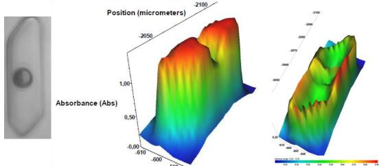
**Figure 4:** Two IR maps (right) of the sampled inclusion (left). The colour relates to the absorbance scale, taken (middle) at the main peak of the OH-stretching band: 3400 cm<sup>-1</sup>, featuring the bulk liquid (e.g. Maréchal, 2007), and (right) at the dangling-OH band: 3680 cm<sup>-1</sup>, characteristic of hydrophobic interfaces (e.g. Miranda and Shen, 1999).
