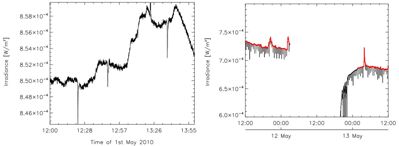
**Fig. 3.** *Left panel:* effects of the Large Angle Rotations of PROBA2 on the channel 4 time series. Periods overlaid in gray indicate data to be removed and have been determined using the housekeeping information plus an algorithm to detect the dips. *Right panel:* in black, the original level 2 data. In red, the data corrected for LARs and slow stabilization after cover opening.
