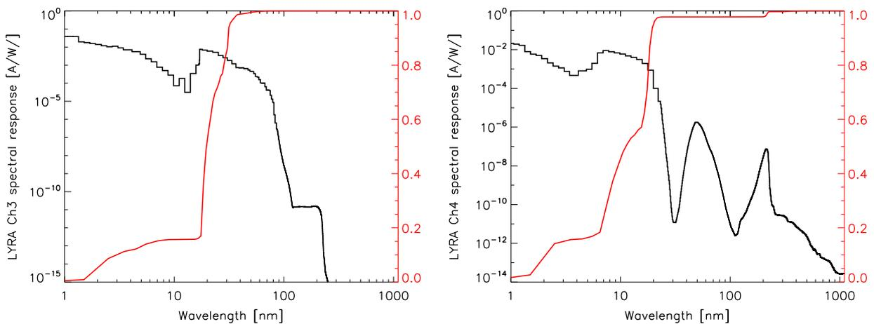
**Fig. 2.** Spectral response of LYRA unit 2 channels 3 (left) and 4 (right). The cumulative spectral contribution has been determined by multiplication of the spectral response by the solar spectrum for 1 February 2010 – quiet solar conditions – as deduced from TIMED/SEE and two instruments aboard the spacecraft Solar Radiation and Climate Experiment: the spectral irradiance monitor (SIM) and the Solar Stellar Irradiance Comparison Experiment (SOLSTICE) (see text for details).
