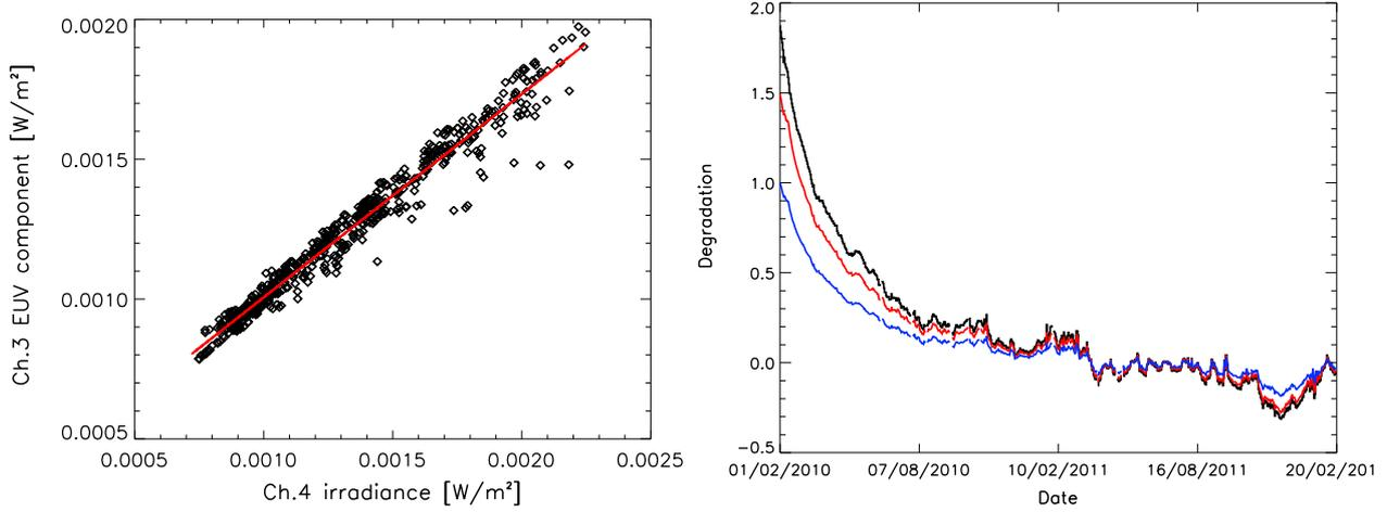
**Fig. 8.** *Left panel:* simulated EUV component of channel 3 vs. simulated channel 4. *Right panel:* the ratio  $L_{\text{Ch3/EUV}}^{\text{deg}}(t)/L_{\text{Ch3/EUV}}^{\text{simu}}(t)$  showing the (multiplicative) degradation of the EUV component. In black,  $L_{\text{Ch3/EUV}}^{\text{simu}}(t)$  has been determined to match the EVE data; in red, to match the TIMED/SEE data; in blue, the normalized curve.
