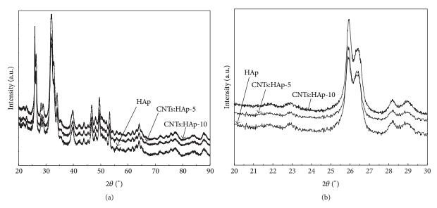
FIGURE 1: Comparative representation of the experimental XRD patterns of the HAp and CNTs:HAp-5 and CNTs:HAp-10 nanocomposites in the  $2\theta$  ranges  $20^{\circ}-90^{\circ}$  (a) and  $20^{\circ}-30^{\circ}$  (b), respectively.
