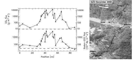
**Figure 10.** Results of the vertical profile in GZ3. A photograph of the profile (taken in 2008) is presented on the right where the location of the ancient cavity is indicated. Results of  $CO_2$  and radon flux measurements are shown on the left as a function of the position along the profile. The horizontal dashed lines correspond to the average background  $CO_2$  and radon fluxes obtained in the SBHS.
