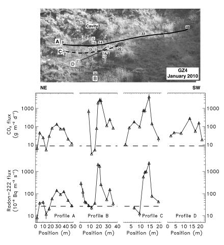
**Figure 11.** Results of the gas measurement profiles A, B, C, and D in GZ4. The photograph (taken in 2010) shows locations of the four profiles and the cavity. The horizontal dashed lines correspond to the average background  $CO_2$  and radon fluxes obtained in the SBHS.
