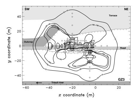
**Figure 14.** Example of estimation of total CO<sub>2</sub> discharge in GZ3. Data points and contours of the CO<sub>2</sub> fluxes expressed in  $g m^{-2} d^{-1}$  are shown. This example yields an estimated total CO<sub>2</sub> discharge of 2.49 ± 0.50 t  $d^{-1}$ . Coordinates (0, 0) correspond to 28.15925°N, 85.33513°E.
