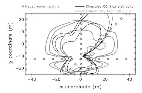
**Figure A1.** Monte Carlo simulation of the estimation of the total discharge using an adaptive strategy with 40 measurement points organized into two perpendicular profiles and one diagonal. The contours of the true discharge  $(2.22 \text{ t d}^{-1})$  are displayed in black while the inferred contours, drawn from interpolating the measured flux, are shown in gray. The obtained total discharge in this case is  $2.28 \text{ t d}^{-1}$ .
