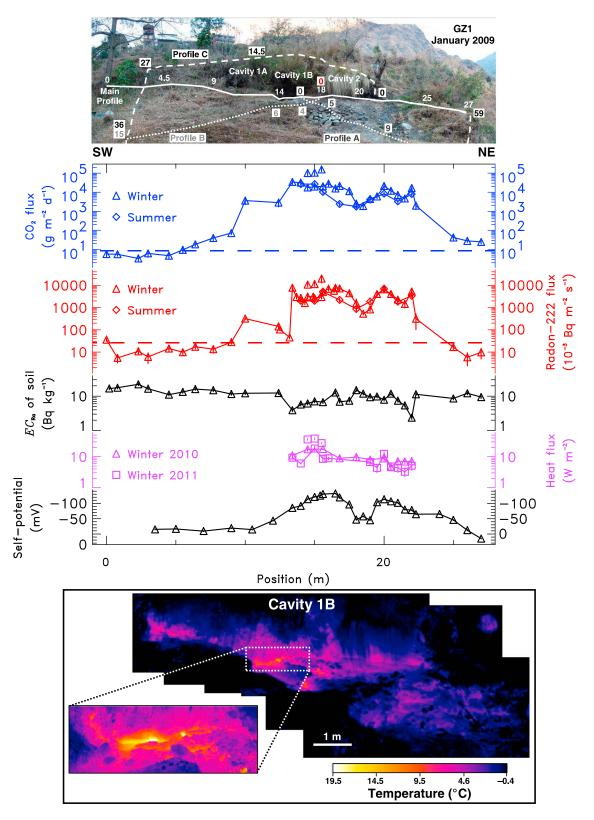
**Figure 6.** Results of the main profile of GZ1. From top to bottom: photograph of the site; results of  $CO_2$  flux, radon flux,  $EC_{Ra}$  of soil samples, heat flux, and SP data as a function of the position along the profile; and thermal infrared image of cavity 1B taken in January 2011. The horizontal dashed lines correspond to the average background  $CO_2$  and radon fluxes obtained in the SBHS.
