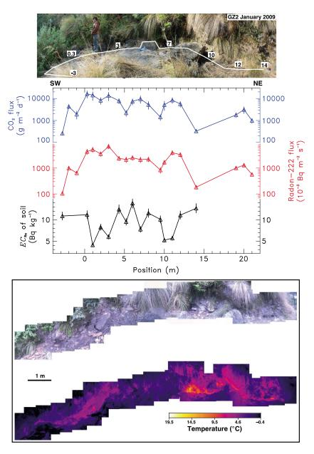
**Figure 8.** Results of GZ2. From top to bottom: photograph of the site; results of  $CO_2$  flux, radon flux, and  $EC_{Ra}$  of soil samples as a function of the position along the profile; and thermal infrared image taken in January 2011. The horizontal dashed lines correspond to the average background  $CO_2$  and radon fluxes obtained in the SBHS.
