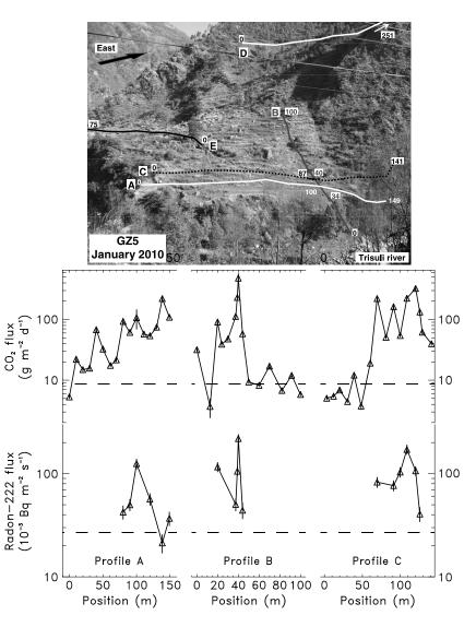
**Figure 12.** Results of the gas measurement profiles A, B, and C in GZ5. From top to bottom: photograph (taken in 2010) of these three profiles together with two background profiles (GZ5D and GZ5E);  $CO_2$  and radon flux results as a function of the position for the three profiles of the gas zone. The horizontal dashed lines correspond to the average background  $CO_2$  and radon fluxes obtained in the SBHS.
