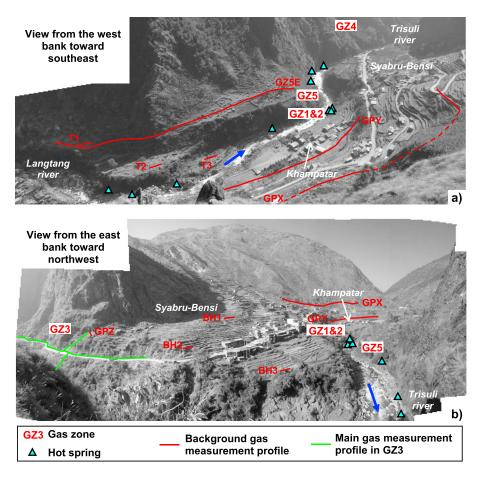
**Figure 2.** View toward (a) southeast and (b) northwest of the Syabru-Bensi hydrothermal system in central Nepal, with the position of hot springs, gas zones, and background gas profiles. Photographs were taken in 2008. The labels GPX, GPZ, GPZ, BH1, BH2, and BH3 on the west bank of the Trisuli River and T1, T2, T3, and GZ5E on the east bank refer to the background gas profiles.
