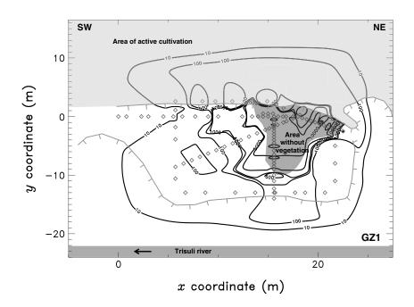
**Figure 13.** Example of estimation of total CO<sub>2</sub> discharge in GZ1. Data points and contours of the CO<sub>2</sub> fluxes expressed in  $g m^{-2} d^{-1}$  are shown. This example yields an estimated total CO<sub>2</sub> discharge of  $1.37 \pm 0.27 t d^{-1}$ . Coordinates (0, 0) correspond to 28.16273°N, 85.33745°E.
