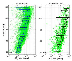
Fig. 2. Altitude distribution of  $SO_2$  mixing ratio from SPICAV UV solar (a) and stellar (b) occultations. Solid lines are weighted mean values with standard deviations. Error bars of individual dots (not shown) are less than the dispersion of the data.
