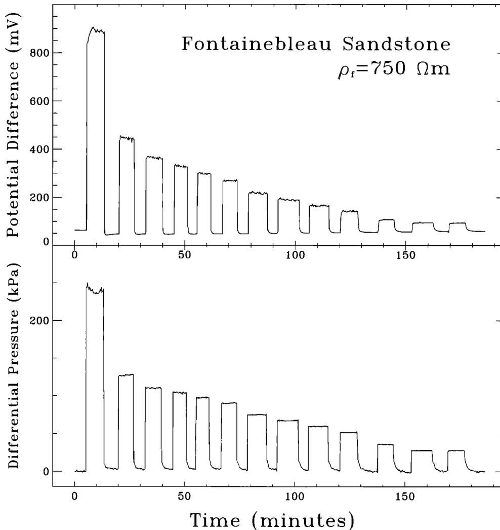
**Figure 4.** A typical streaming potential measurement with Fontainebleau sandstone. The electric potential reference is taken at the high-pressure end (convention of *Morgan et al.* [1989]). A positive potential difference (i.e., a positive streaming potential coefficient) corresponds to a negative  $\zeta$  potential. A single measurement of streaming potential takes  $<10$  min to reach a stable value. The electrode drift during that time is in general  $<1$  mV.
