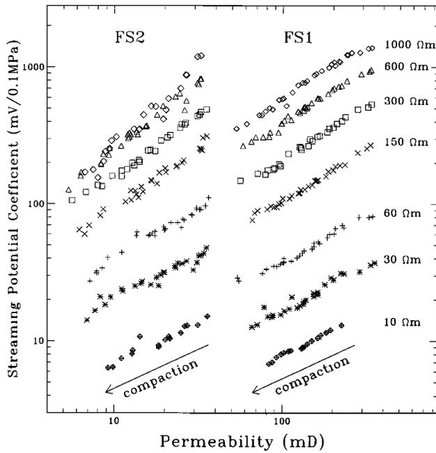
**Figure 13.** Streaming potential coefficient as a function of permeability for various electrolyte resistivities during compaction for Fontainebleau sandstone samples FS1 and FS2. The experimental errors are given by the size of the symbols.
