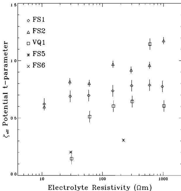
**Figure 17.** The permeability exponent  $t$  parameter of the effective  $\zeta$  potential versus electrolyte resistivity during compaction ( $\zeta_{\text{eff}} \sim k'$ ) for Fontainebleau sandstone and Villejust quartzite samples.
