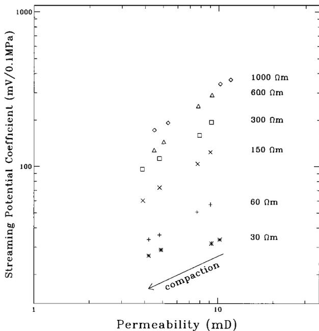
**Figure 14.** Streaming potential coefficient as a function of permeability for various electrolyte resistivities during compaction for Villejust quartzite sample VQ1. The experimental errors given by the size of the symbols.
