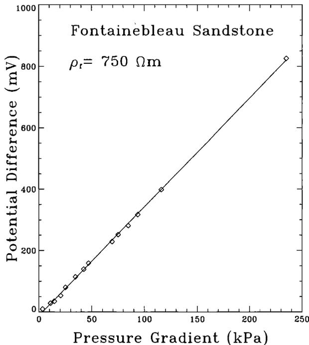
**Figure 5.** Potential difference as a function of the pressure gradient for the experiment shown in Figure 4. The experimental errors are of the order of the size of the symbols. This experiment yields a positive streaming potential coefficient of 350 mV/0.1 MPa.
