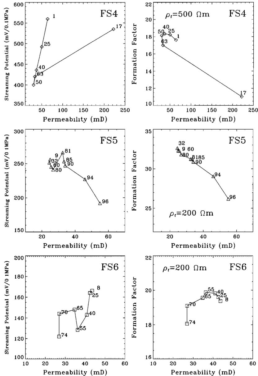
**Figure 19.** Streaming potential coefficient and formation factor during uniaxial compression and rupture for three Fontainebleau sandstone samples. The number indicated near each data point corresponds to the value of the uniaxial force. The values of the electrolyte resistivity were  $500 \Omega m$  for FS4 and  $200 \Omega m$  for FS5 and FS6.
