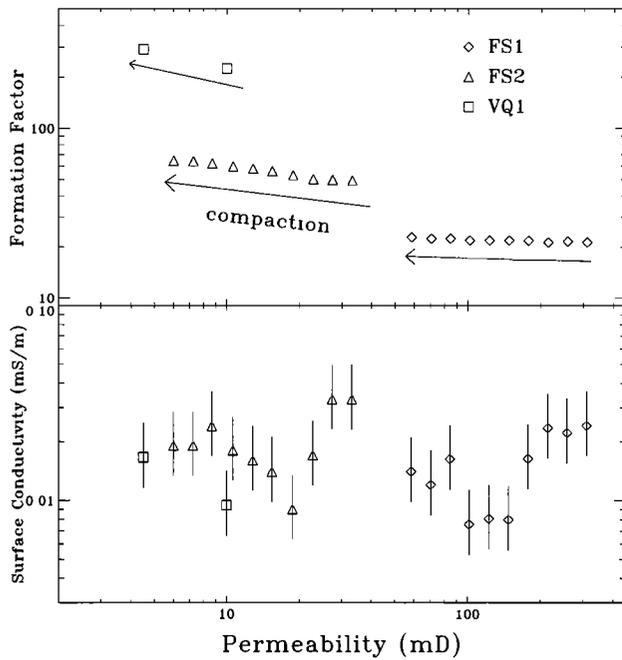
**Figure 12.** Bulk formation factor and surface conductivity as a function of permeability for three rock samples during compaction. The experimental error on the values of the formation factors is indicated by the size of the symbols.
