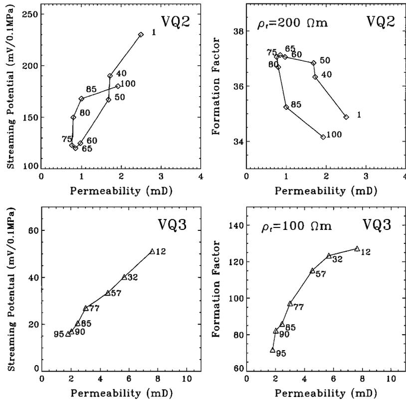
**Figure 20.** Streaming potential coefficient and formation factor during uniaxial compression and rupture for two Villejust quartzite samples. The number indicated near each data point corresponds to the value of the uniaxial force. The values of the electrolyte resistivity were  $200 \Omega\text{m}$  for VQ2 and  $100 \Omega\text{m}$  for VQ3.
