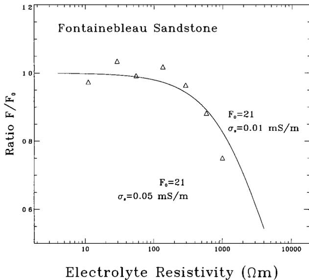
**Figure 8.** The streaming potential correction factor  $F/F_0$ , as derived from the measurements of rock and electrolyte conductivity measurements for one sample of Fontainebleau sandstone (Figure 7). The full line corresponds to the calculated value assuming a bulk formation factor of 21 and a surface conductivity of 0.01 mS/m. The dotted line corresponds to the calculated value assuming a bulk formation factor of 21 and a surface conductivity of 0.05 mS/m.
