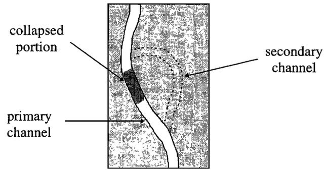
**Figure 18.** A simple model for the evolution of transport properties associated with pore collapse during compaction. When the shaded portion collapses, fluid percolation proceeds through a secondary path.
