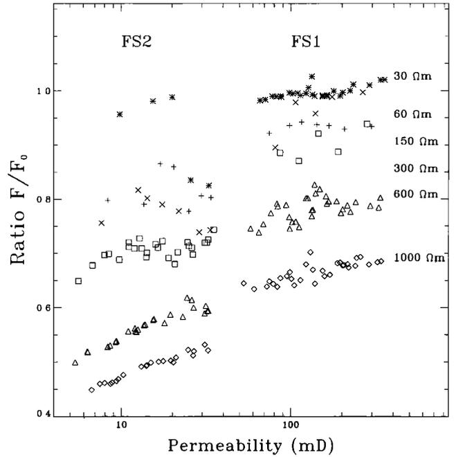
**Figure 15.** The ratio  $F/F_0$ , determined using equation (10), as a function of permeability for various electrolyte resistivities during compaction for Fontainebleau sandstone samples FS1 and FS2.
