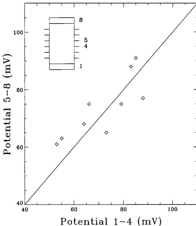
**Figure 6.** The potential difference between disk electrode 1 and ring electrode 4 compared with the potential difference between ring electrode 5 and disk electrode 8. The position of the electrodes is shown. The various measurements corresponds to several steps during the uniaxial deformation of the sample.
