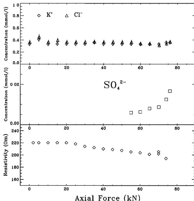
**Figure 22.** Concentrations of K<sup>+</sup>, Cl<sup>-</sup>, and SO<sub>4</sub><sup>2-</sup> ions and the electrolyte resistivity (coming out of the sample, see Figure 3) during rupture of Fontainebleau sandstone sample FS6, as a function of the uniaxial force. The ion concentrations are measured by capillary electrophoresis and have an uncertainty of 10%.
