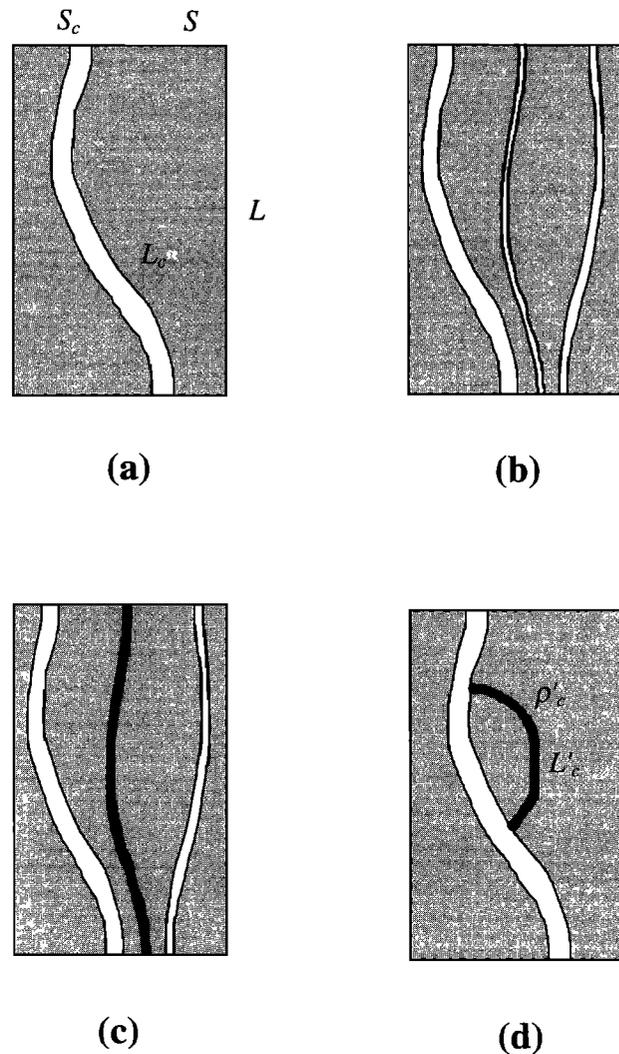
**Figure 1.** Various flow patterns in capillary tubes in a non-conducting matrix: (a) one single capillary (equivalent channel), (b) distribution of capillary tubes of various diameters and tortuosities, (c) distribution of capillaries including some containing a nonflowing conducting medium (in black), and (d) capillary tube with a branch containing a nonflowing conducting medium.
