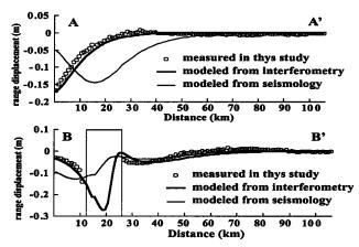
Figure 3. Comparison between ground displacements along the radar line of sight. 1) measured from unwrapped interferogram, 2) computed from the seismological model [*Klinger et al.* 1999] and 3) modeled in this study. See Figure 2c for location of profiles. Gray box denotes location of the gulf.
