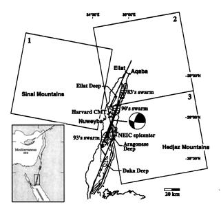
Figure 1. Seismotectonic map of the Gulf of Aqaba adapted from *Ben Avraham* [1985]. Dashed areas show extent of 1983, 1990 and 1993 seismic swarms. Stars represent epicenter and centroid. The trace at the bottom of the gulf of the best fault segment modeled in this study (black segment), and associated focal mechanism (see Table 2) are indicated. Black boxes depict location of interferograms.
