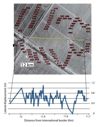
**Figure 8.** Offset crop rows between 11.7 and 12 km northwest of the international border. Crops rows could be measured to 10–15 cm of resolution because they had recently been planted and were not yet mature, but offsets vary by more than 1 m. The color version of this figure is available only in the electronic edition.
