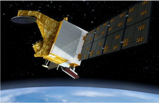
Figure 1. Artist view of the CFOSAT satellite. The SWIM antenna system is on the left. It is composed of a rotating plate with 6 feed-horns and an offset parabolic antenna. The SCAT antenna system is on the bottom right. It is a set of two opposed plane antenna. Other antennas on Earth face are for TM/TC (X and S-bands).. © CNES/ Gekko.
